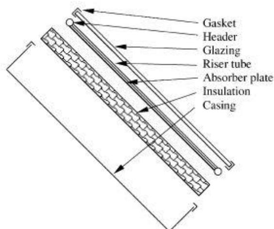
**Fig (I-5):** Exploded view of a flat-plate collector.
