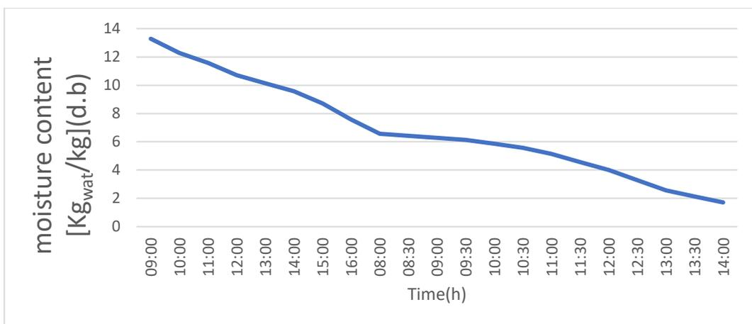
**Fig (IV-2e):**Variation moisture content (d.b) in natural drying
