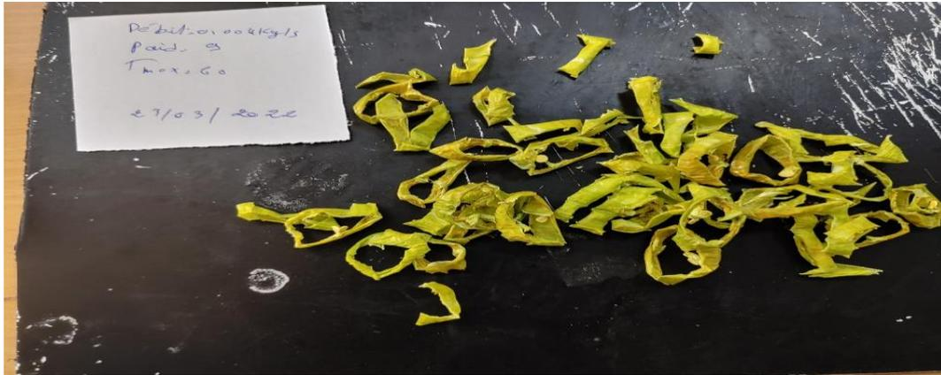
**Fig(III-8):** Green chili after drying in oven drying in 60 °c with flow=0.004kg/s
