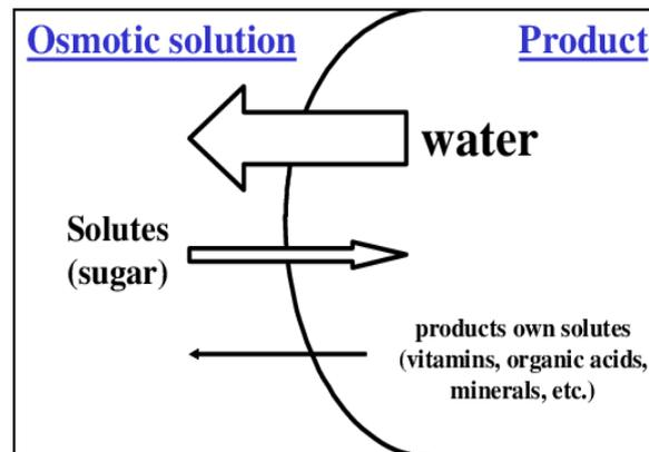
**Fig(I-2):** Principle of the osmotic dehydration.
