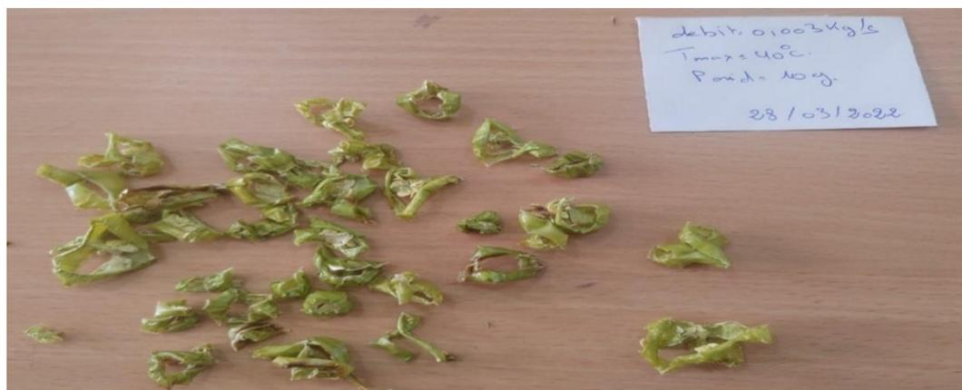
**Fig (III-13):**Green chili after drying in oven drying in 40 °c with flow=0.003kg/s
