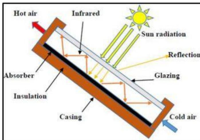
Fig (I-6): Principle of solar heat collector.
