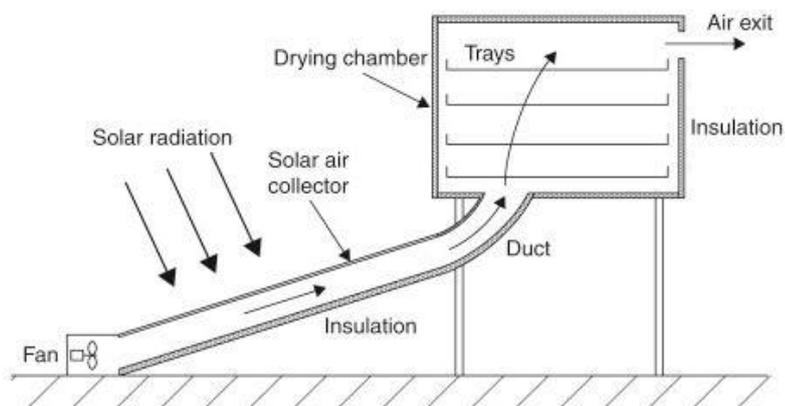
**Fig (I-11):** Principe indirect solar drying
