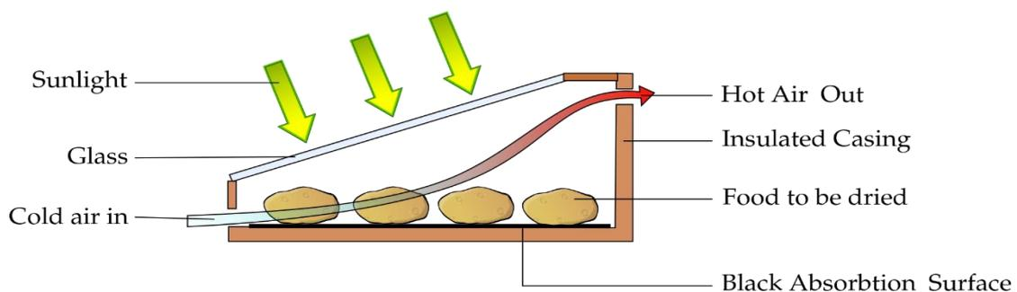
Fig (I-9) : Principe direct solar drying
