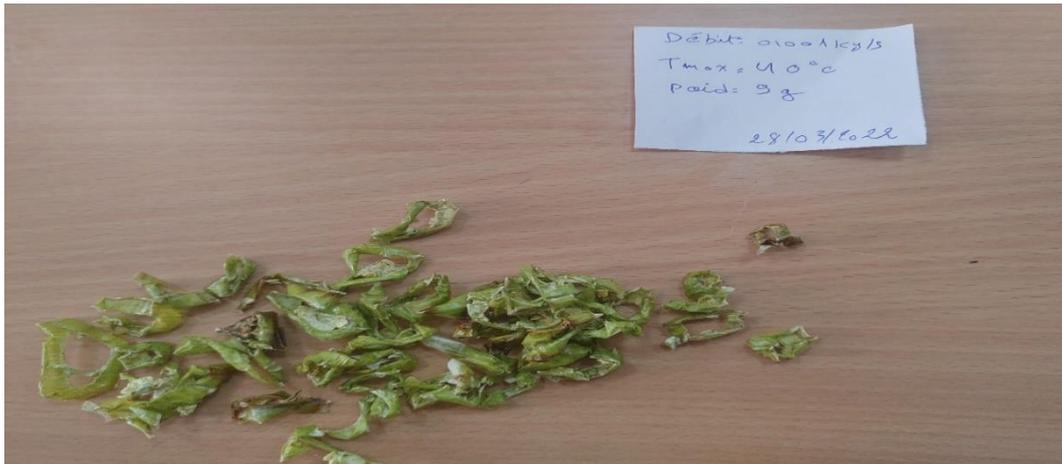
**Fig (III-14):**Green chili after drying in oven drying in 40 °c with flow=0.001kg/s
