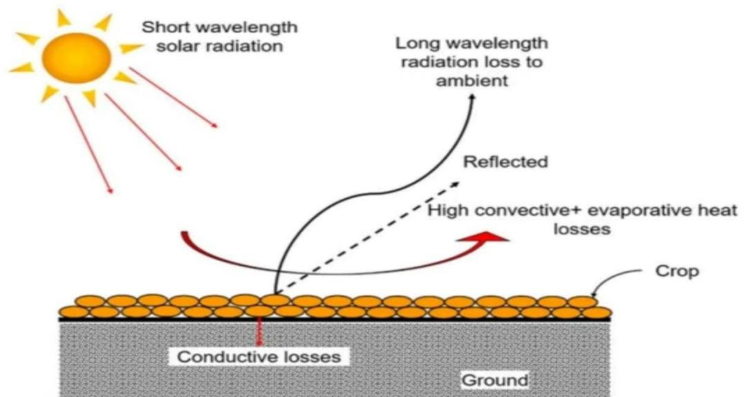
**Fig (I-8):** Principle of sun drying
