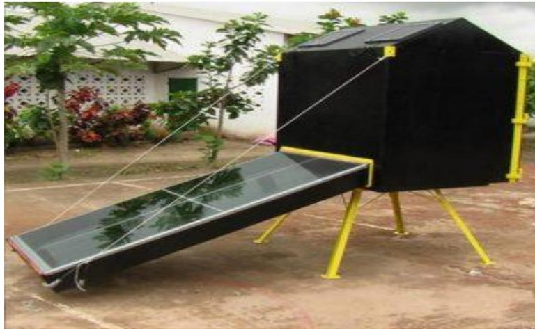
**Fig (I-10):** Indirect solar drying
