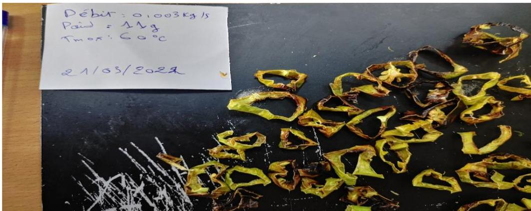
**Fig (III-9):** Green chili after drying in oven drying in 60 °c with flow=0.003kg/s
