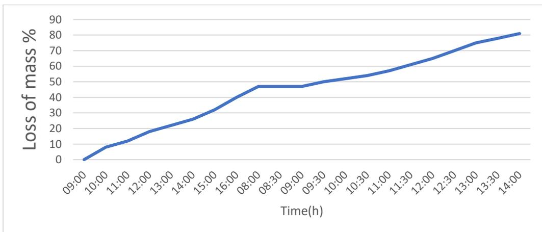
**Fig (IV-4e):** Variation Loss of mass in natural drying
