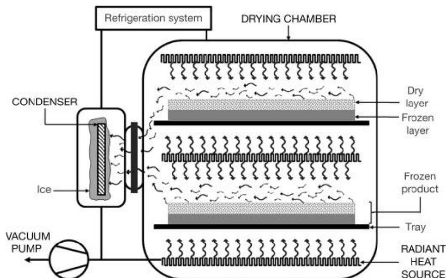
**Fig(I-1):** Freeze dryer diagram.
