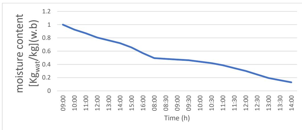
**Fig (IV-3e):**Variation moisture content (w.b) in natural drying
