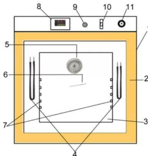
Fig (I-4):Drying oven diagram
