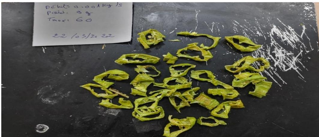
**Fig (III-10):** Green chili after drying in oven drying in 60 °c with flow=0.001kg/s
