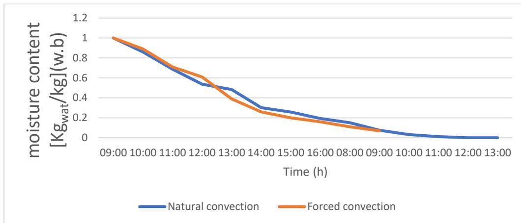
**Fig (IV-3d):**Variation moisture content content(w.b) solar drying
