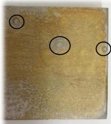
**Figure IV.1:** Pitting Corrosion
