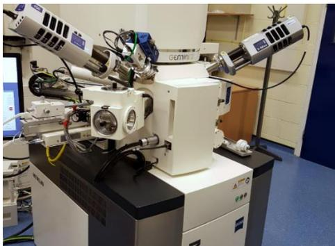
**Figure III.7:** Scanning Electron Microscope (SEM) <sup>[62]</sup>.
