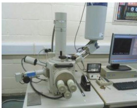
**Figure III.8:** Energy Dispersive X-Ray Analysis <sup>[64]</sup>.
