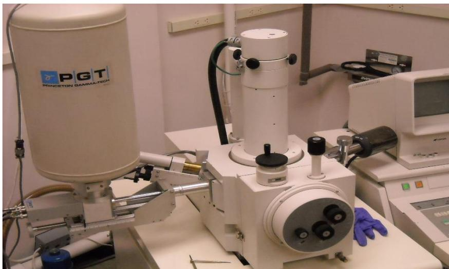
**Figure II.15:** Energy Dispersive X-Ray Analysis (EDX) <sup>[58]</sup>.
