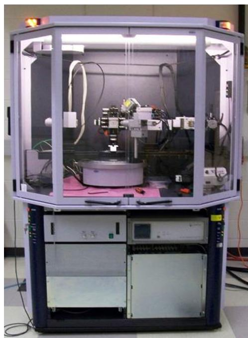
**Figure III.9:** X-ray diffraction studies<sup>[66]</sup>.
