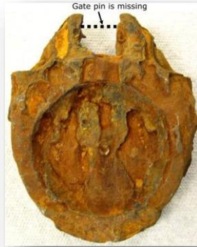
**Figure I.1:** Uniform Corrosion <sup>[7]</sup>.
