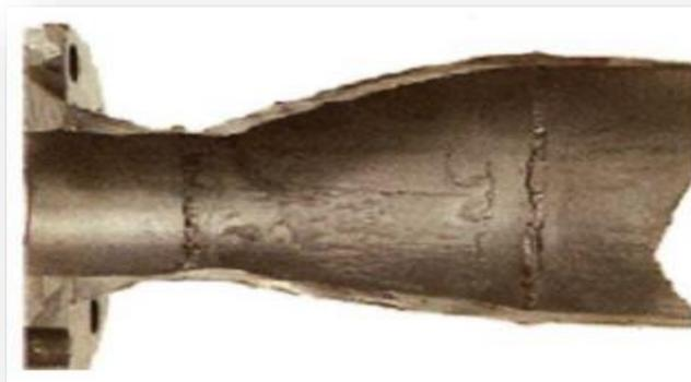
**Figure I.5:** Corrosion-erosion in turbulent areas<sup>[13]</sup>.
