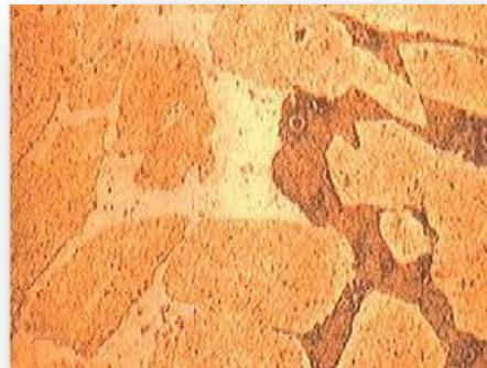
**Figure I.7:** Mechanism of selective corrosion of a brass (copper-zinc alloy).
