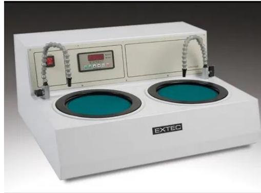
Figure III.2: The polishing machine <sup>[60]</sup>.
