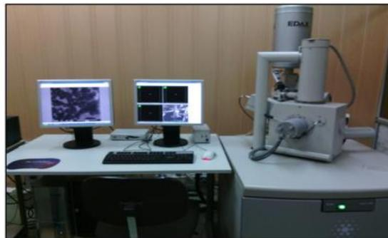
**Figure II.10:** Scanning Electron Microscopy Apparatus (SEM) <sup>[52]</sup>.
