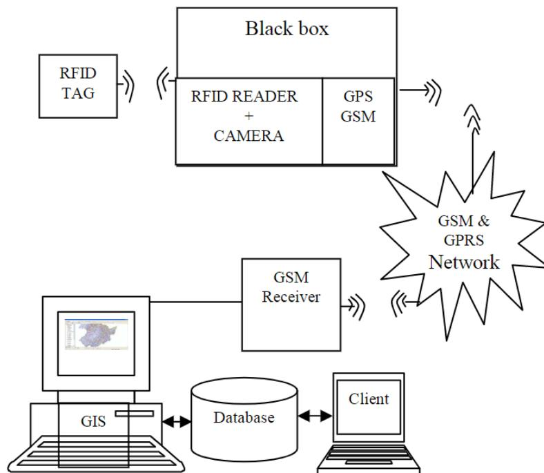
Figure II.1: Architecture of waste monitoring system
