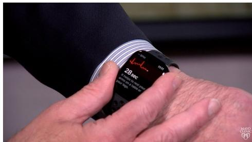
Figure 1.1 – ECG signals generated from the single lead on an Apple Watch.
