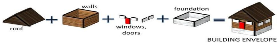
Figure 1. Architectural envelope components
