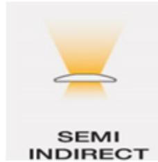
Figure 35 Semi indirect lighting scheme
