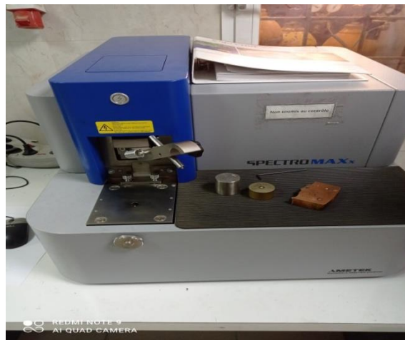
Figure III.19: Photo of the Spectro-MAXx Analysis
