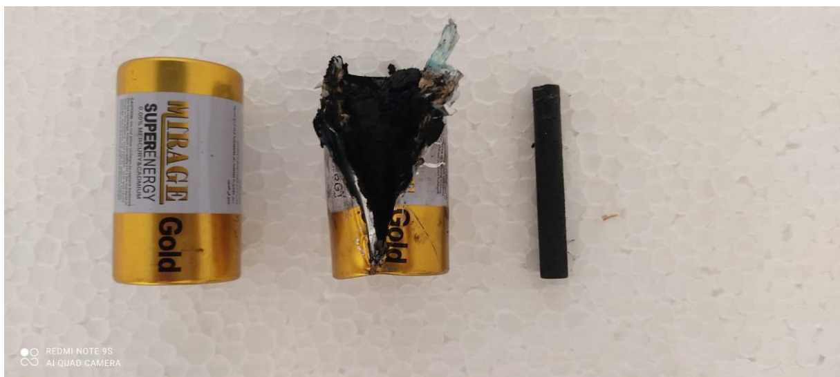
Figure III.13: Graphite electrode extracted from batteries
