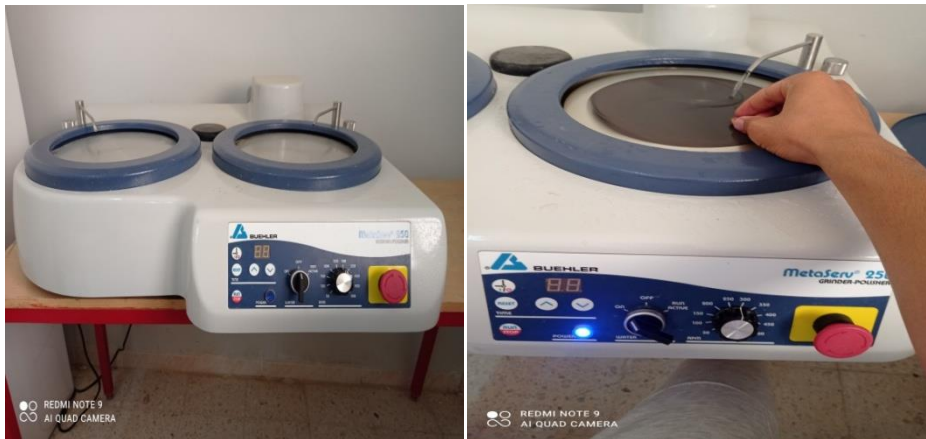
Figure III.18: Mechanical polishing process
