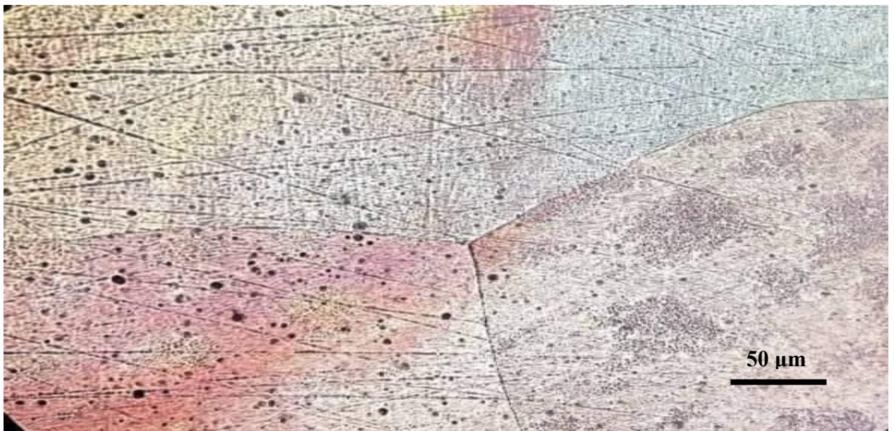
Figures III.22: The microstructure of the melted sample (C40%, D260%)
