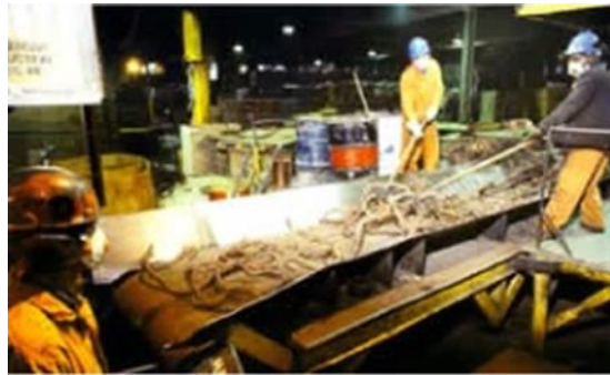
Figure I.3: Feeding recovered copper wire into a conveyor belt for recycling [2]
