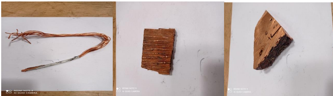
Figures III.1: copper waste 1 (W1) Figures III.2: Copper cathode (C) Figures III.3: copper waste 2 (W2)
