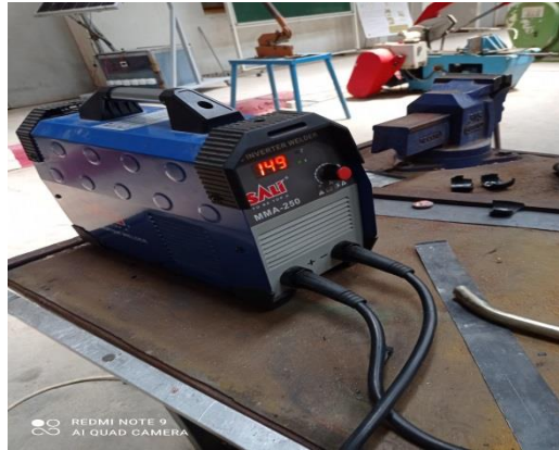
Figures III.12: Inverter welding machine type SALI MMA-250
