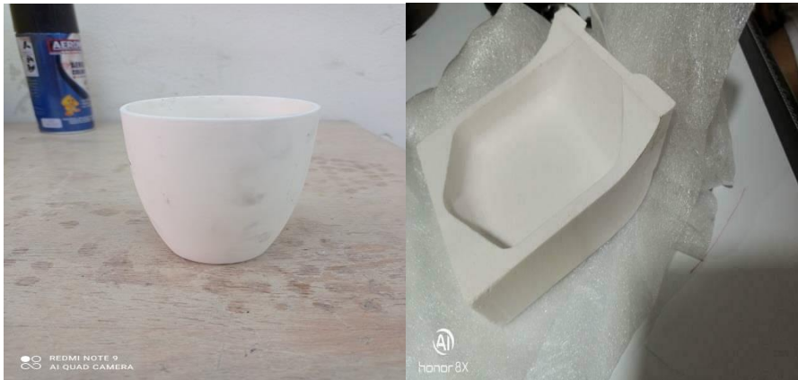
Figures III.5: Shape of Refractory used in smelting
