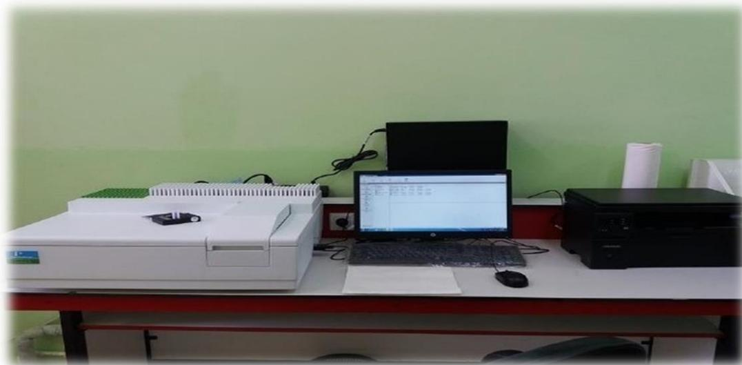
**Figure 8** : UV/VIS spectrophotometre
