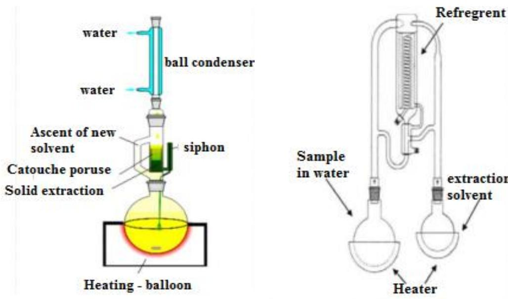
**Figure 9:** Soxhlet apparatus on the left, and Lickens-Nickerson apparatus on the right.
