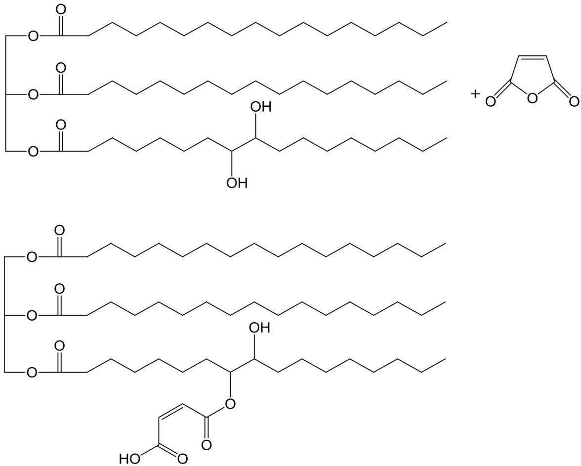
**Figure 31:** Esterification of hydroxylated oils with maleic anhydride.
