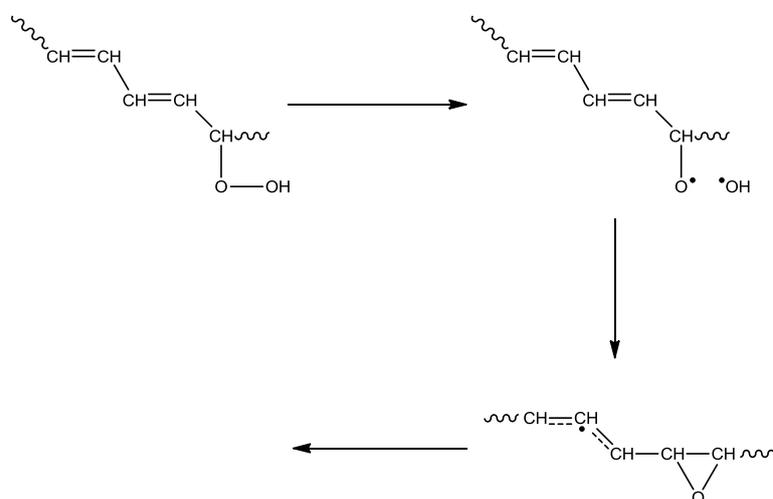
**Figure 4:** Epoxy formation by reaction of hydroperoxides on double bonds.
