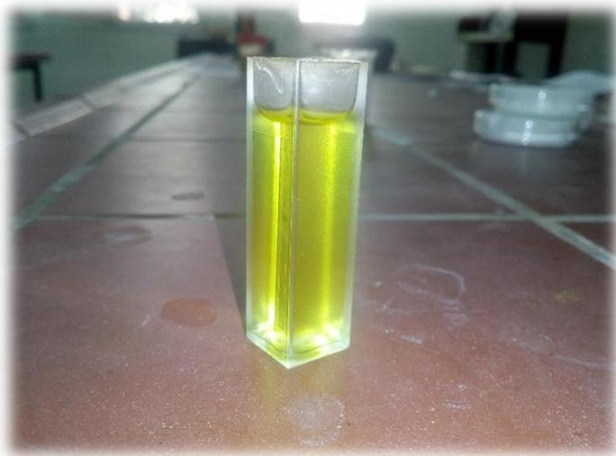
Introduce the cuvette into the spectrophotometer and close the hood:
