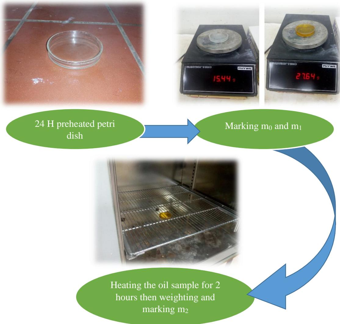
**Figure 5:** water rate measuring protocol
