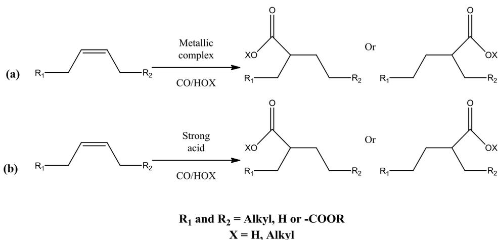
**Figure 14:** Hydroxycarboxylation reaction (a) and Koch reaction (b) for the introduction of a carboxylic acid function on the double bonds of vegetable oils [69].
