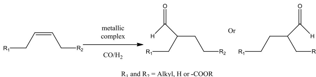
**Figure 13:** Hydroformylation reaction on vegetable oil unsaturations.
