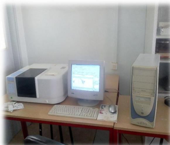
Finally you get to perform your FTIR analysis by launching the specified software (Shimadzu IR Solution) via PC and you get your spectrum.
