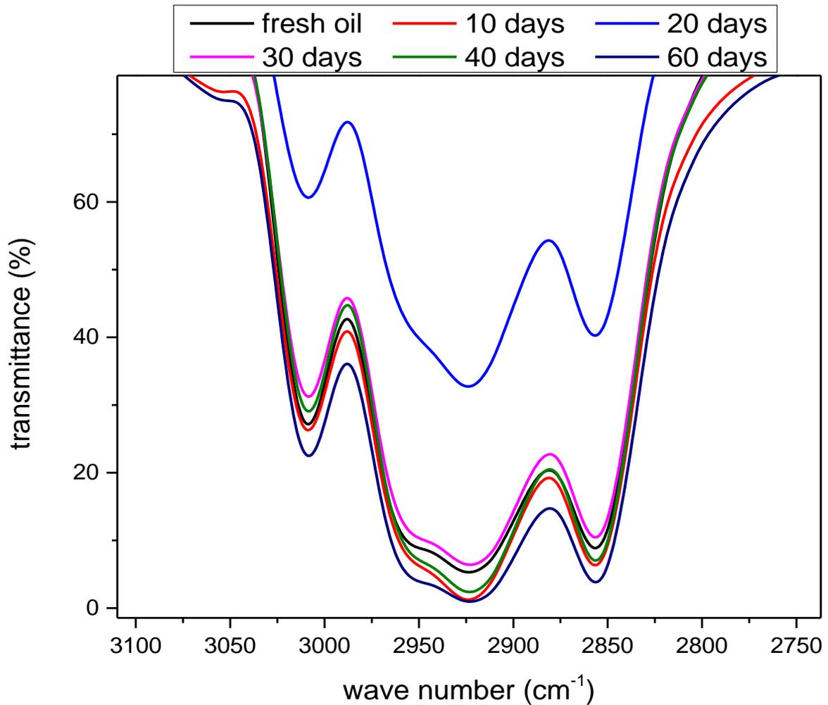
**Figure 9:** CH<sub>2</sub>/CH<sub>3</sub> intensity evolution between 3000-2840 cm<sup>-1</sup> (Zoom of Figure 5)
