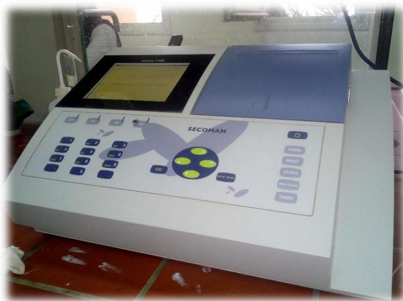
**Figure 9:** UviLine 9400 SECOMAM UV spectrophotometer
