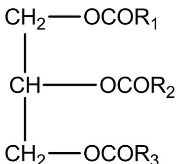
R<sub>1</sub>, R<sub>2</sub>, R<sub>3</sub> are long alkyl chains (in most of fatty acids, C<sub>12</sub>, C<sub>14</sub>, C<sub>16</sub> or C<sub>18</sub> saturated or not). Triglycerides are homogeneous, it means that R<sub>1</sub> = R<sub>2</sub> = R<sub>3</sub> or mix because R<sub>1</sub>, R<sub>2</sub>, R<sub>3</sub> are different. Many fatty acids enters in the composition of each oil and the triglycerides are the most found mixes.
