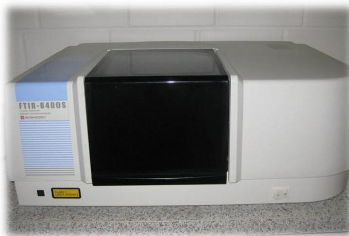
**Figure 8:** FTIR-8400 S Shimadzu infrared spectrophotometer
