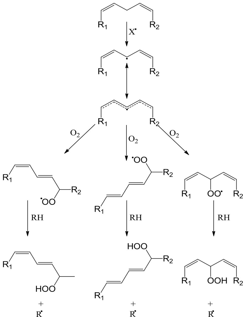
**Figure 13:** Hydroperoxides formation mechanism.
