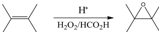
**Figure 10:** Epoxidation method for vegetable oils using hydrogen peroxide [55].
