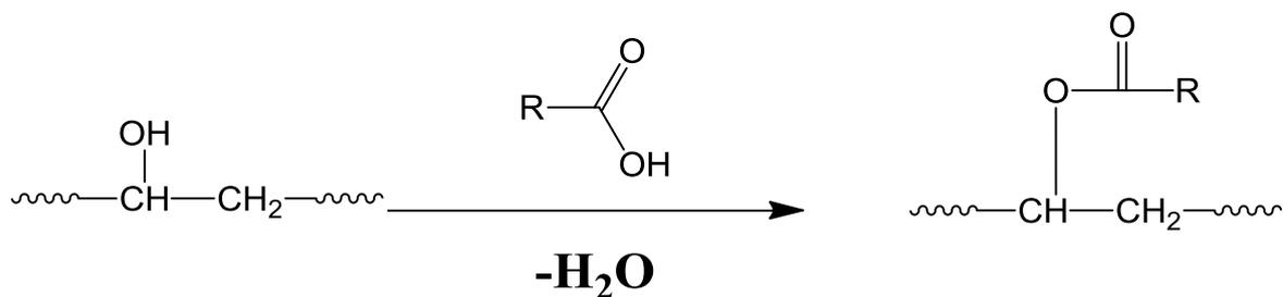
**Figure 30:** Esterification of oils from hydroxyl functions of fatty acid chains.
