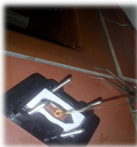
Close the support and introduce it to the spectrophotometer:
