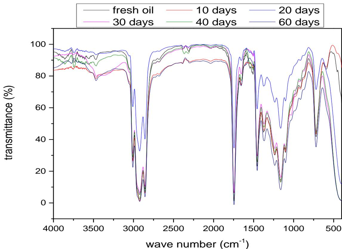
**Figure 5:** FTIR spectrum of linseed oil exposed to air and sun
