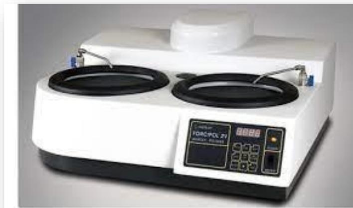
**Figure (III.3):** The polishing apparatus (polisher).
