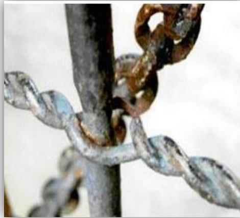
**Figure (I.10):** Schematic representation of Fretting corrosion.
