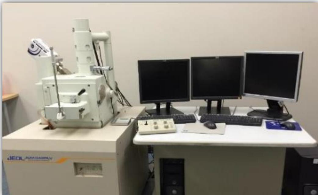
**Figure (II.12):** Photograph of the scanning electron microscope.
