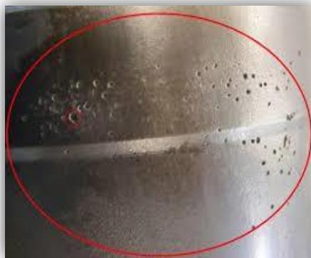
**Figure (I.11):** Schematic representation of Cavitations corrosion.
