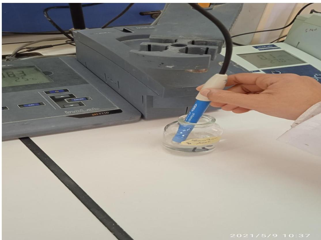
**Figure 3.** pH meter (pH 7110) (original photo)
