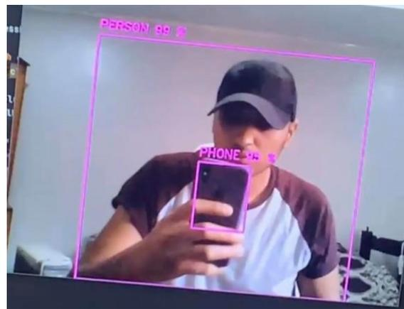
Example of the Object Detector node working in real-time (yolov4)
