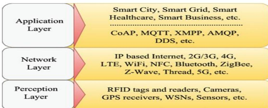
**FIGURE 1.1.** The layers of IoT architecture. [12]
