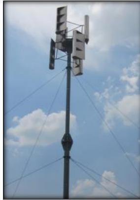
**Figure 2.6:** Prototype of the proposed Senegal VAWT.[18]
