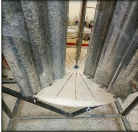
Figure 3.22: Fifteen blades perpendicular to each other three by three.
