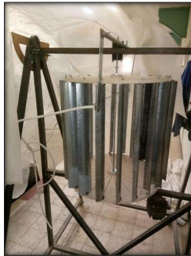
**Figure 3.2:** Fabricated model of quart-circular rotor montage H (twenty bladed).
