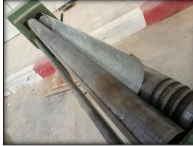
**Figure 3.1:** fabricated quarter- circular bladed.
