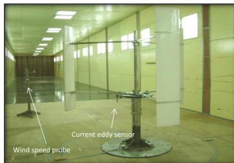
**Figure 2.12:** Wind turbine model installed in the wind tunnel.[21]
