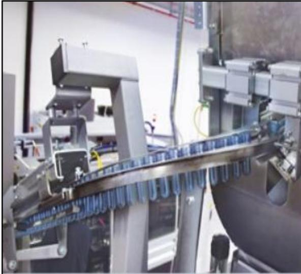
**Fig II.4** :Alimentation des préformes
