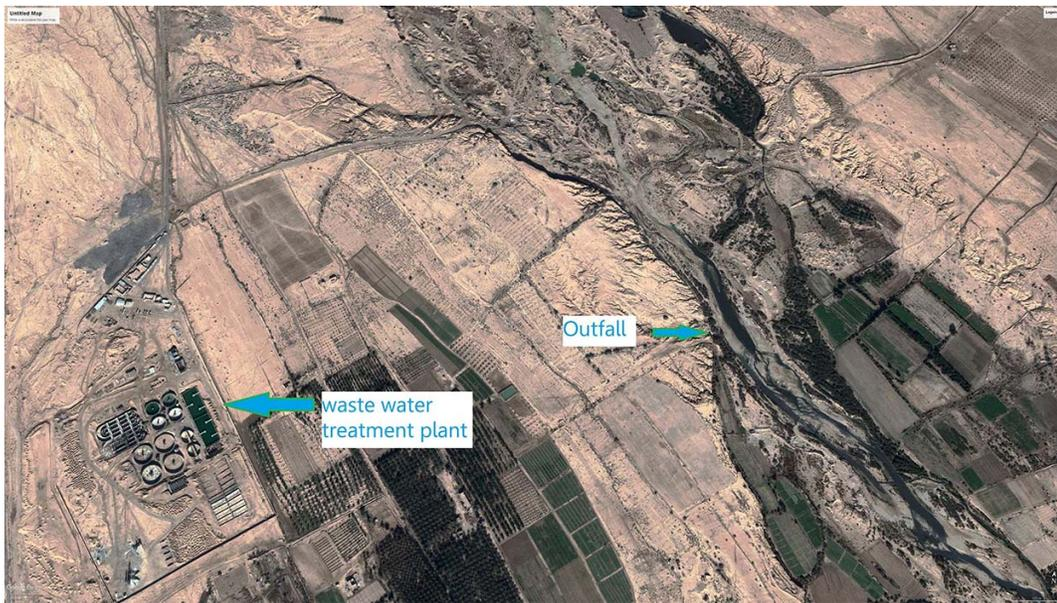
Figure 3.2: An aerial view of the wastewater outfall of the city of Biskra
