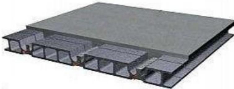
**Figure I.1:plancher a corps creux**
