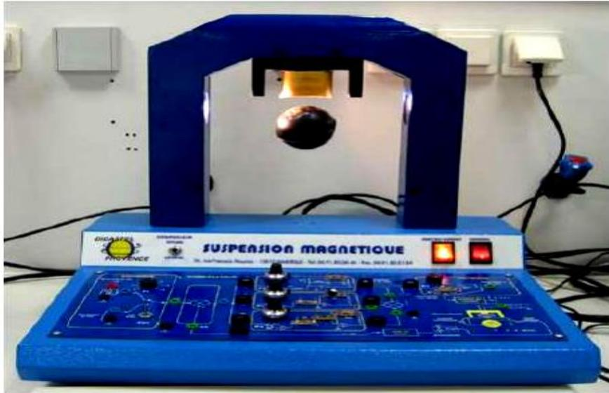
Figure 3.12 :Didastel magnetic suspension (Maglev unit)
