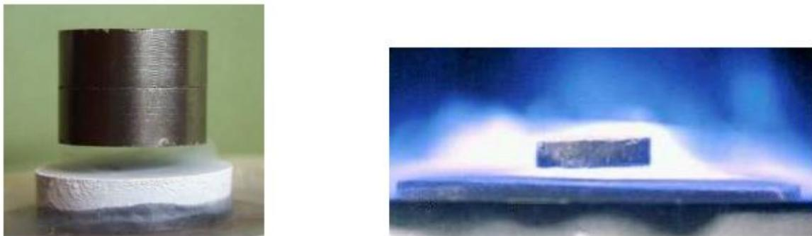
**Figure 1.3 : A magnet floats above a superconductor**
