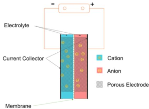
Figure 1.9: Schematic illustration of a supercapacitor[19]
