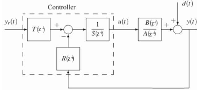
Figure 2.6: Structure of RST controller[14]
