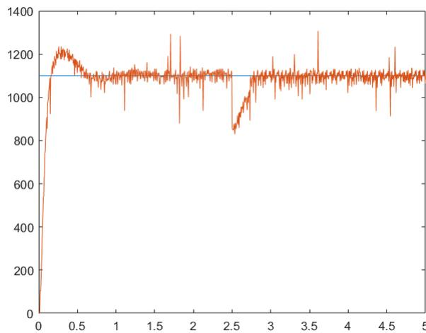
(b) 1100 Rpm ,  $Tr=0.4825Nm$
