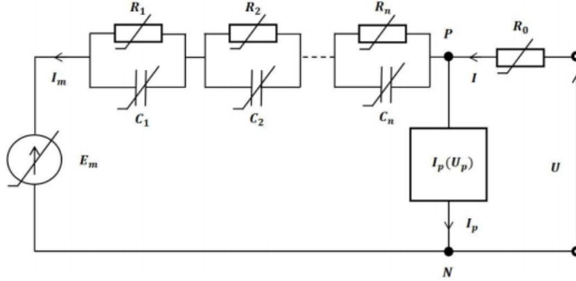
Figure 2.1: Electric diagram of the lead-acid battery cell[4]
