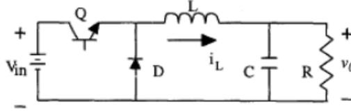
Figure 2.3: DC-DC Buck Converter[10]
