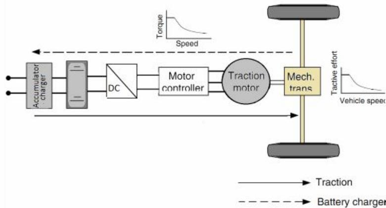
Figure 1.6: Pure electric vehicle [11]
