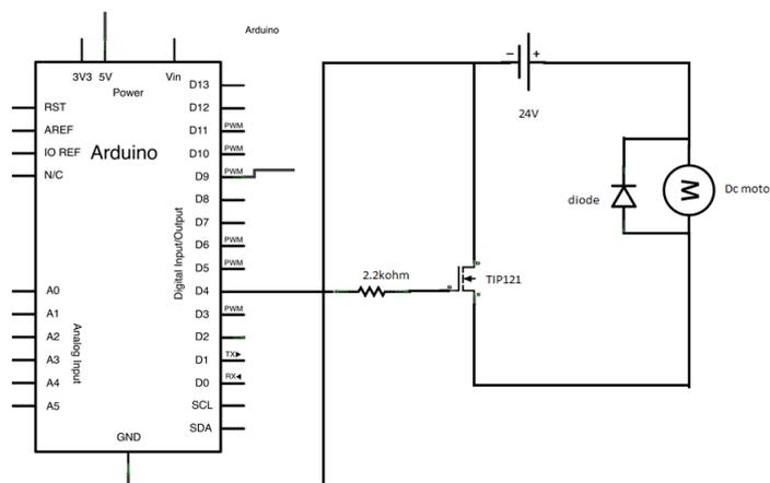
Figure 3.1: A Diagram of the Experimental Circuit
