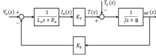
Figure 2.2: Block diagram of DC motor armature control
