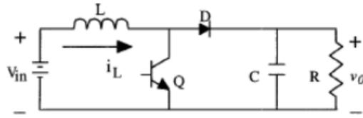
Figure 2.4: DC-DC Boost Converter[10]
