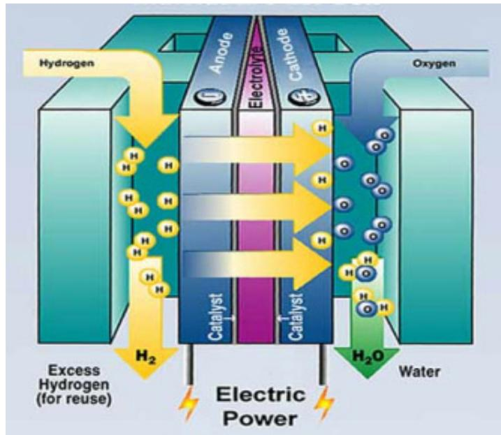
Figure 1.8: Concept of a fuel cell[8]
