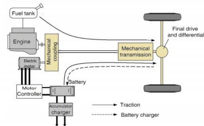
Figure 1.4: Parallel hybrid vehicle [11]
