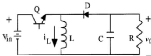
Figure 2.5: DC-DC Buck-Boost Converter[10]
