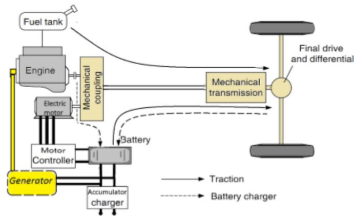
Figure 1.5: The dual mode hybrid vehicle [11]
