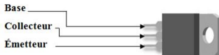
Figure C.2: Transistor TIP121
