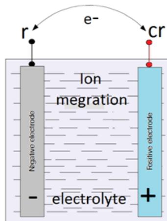
Figure 1.7: An electrochemical battery cell
