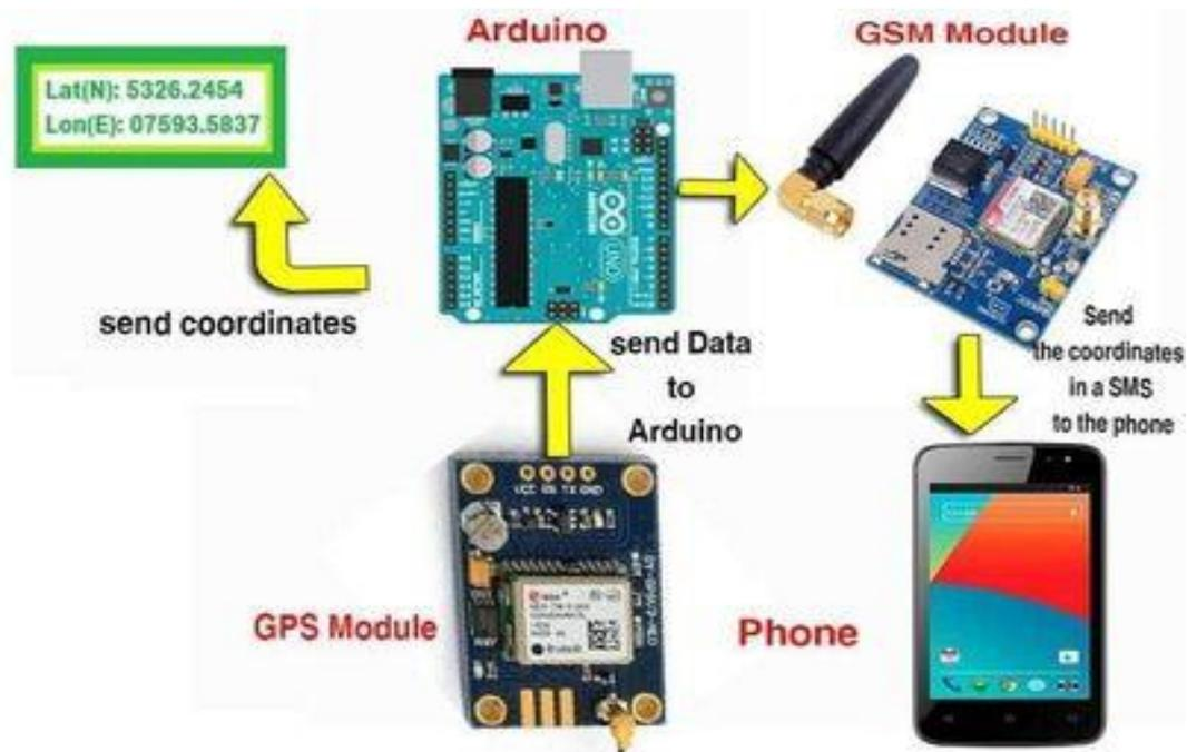
Figure III. 1 The block diagram of GPS tracking system
