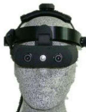
**Figure 6: Head Mounted Display**
