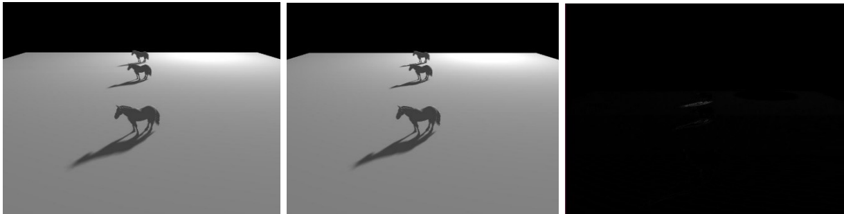
Figure. 3.14. Visual comparison between our result and the reference image. Left image: the proposed technique with 29 rendering passes and with multiple PCF (0.29 seconds). Image in the middle: image acting as Ground Truth with 256 rendering passes (4 seconds). Right image: difference image between the Ground Truth image and the image generated by the proposed technique.
