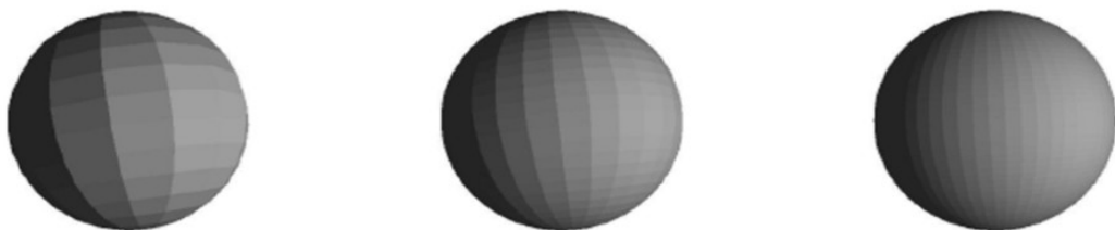
Figure 1.8. Flat shading of the sphere for 16 \times 16 facets, 32 \times 32 and 64 \times 64 [Fra02].
