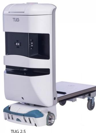
Figure 1.7: The TUG system transports a variety of hospital carts. It automates and tracks the delivery of goods in hospitals [21].
