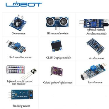
Figure 2.3 – Different Robot sensors
