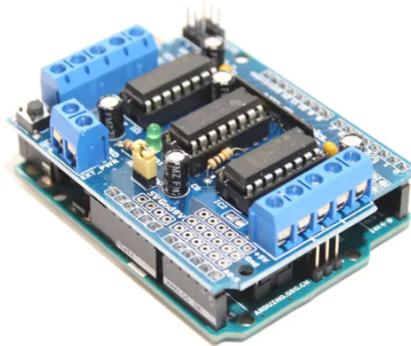
Figure 4.18 – L293D Motor Driver Shield
