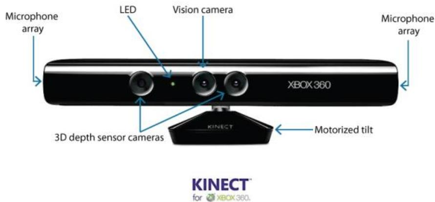
Figure 3.3: the depth sensors of camera Kinect.
