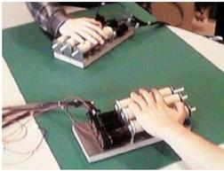
We then present InTouch, which applies Synchronized Distributed physical object to create a “tangible telephone “for long distance haptic communication. Scott brave and Professor Hiroshi Ishii.
