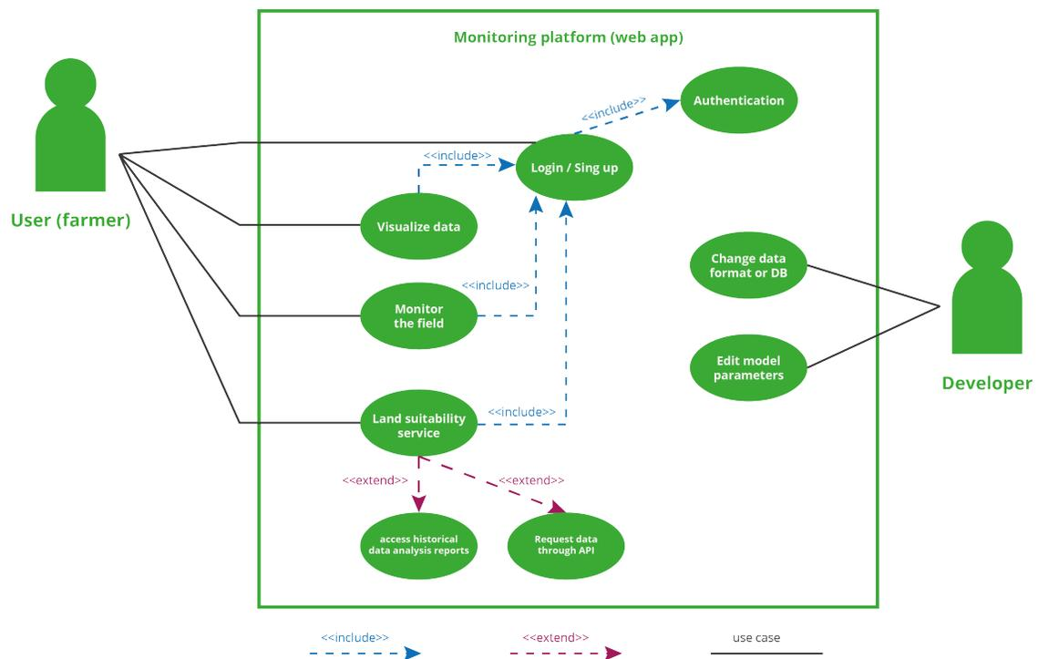
Figure 4.7: Use case diagram of the platform
