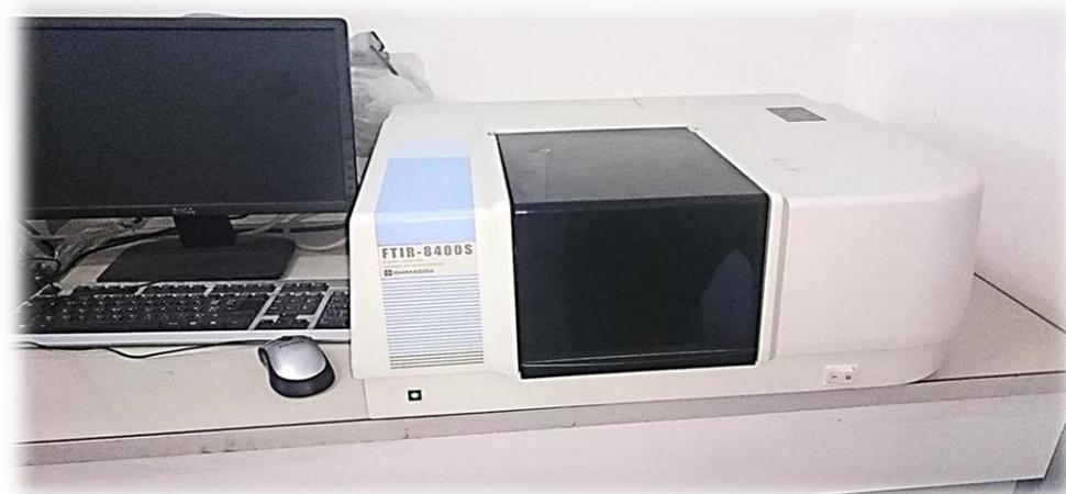
**Figure I.8.** IR spectroscopy dispositive.
