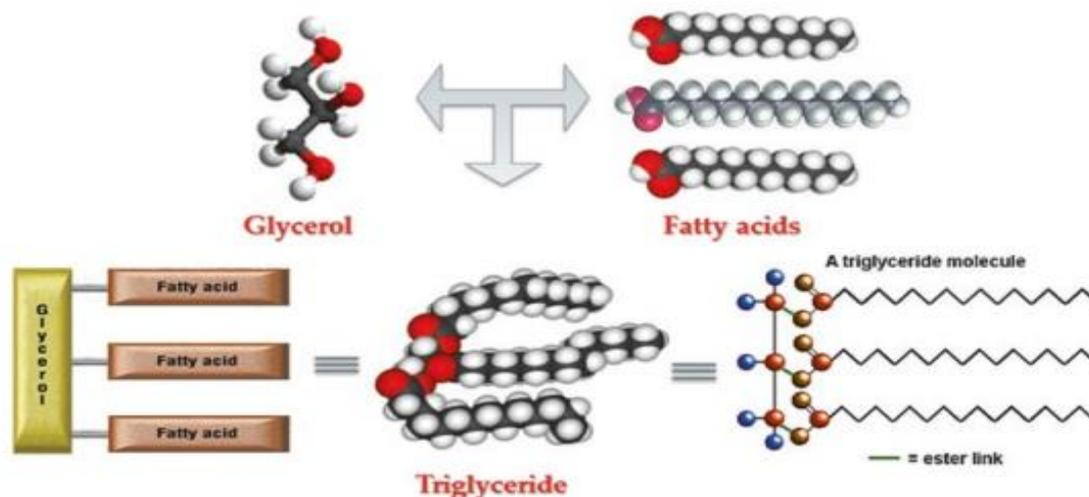
**Figure II.2:** Chemical structure of Triglyceride (natural esters)
