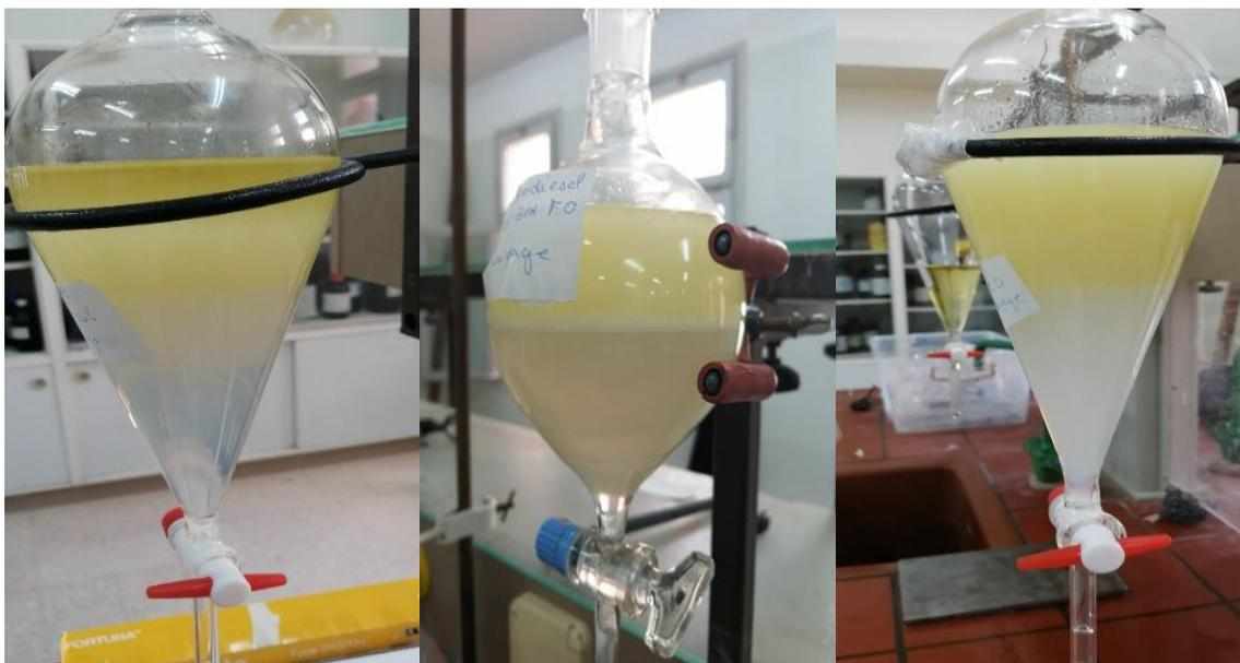
**Figure III.12:** Experimental examples of washing up step with biodiesel new oil, biodiesel 3<sup>rd</sup> frying oil and biodiesel 6<sup>th</sup> frying oil
