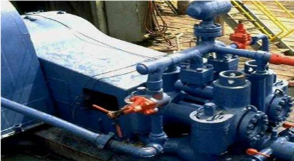
**Figure II.12:** pompe duplex double effet.
