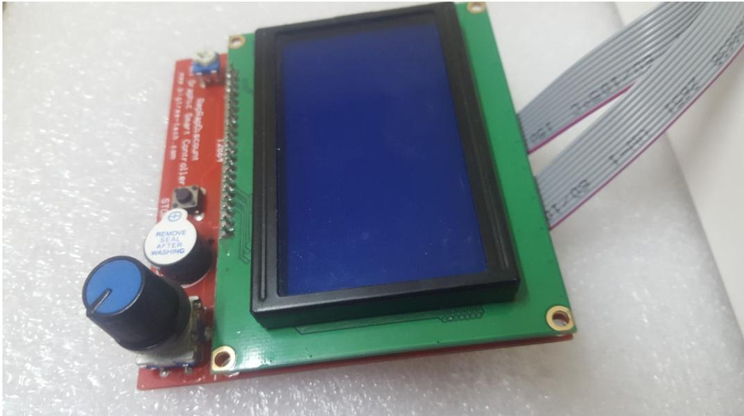
Figure 3.8: 3D Printer LCD display controller
