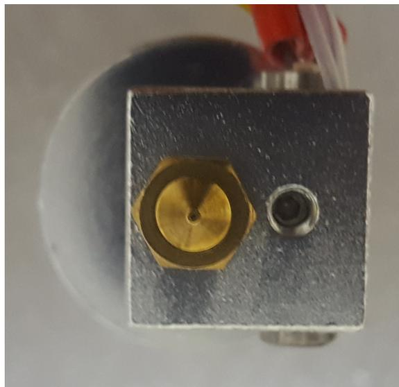
Figure 3.7: Printing head bottom view
