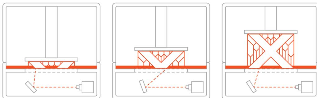
Figure 1.5: 3D printing process VAT Photopolymerisation based [[All19](#)]
