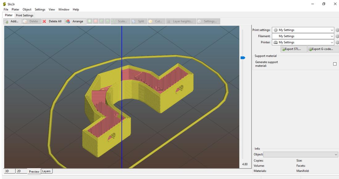
Figure 4.38: before final layer for the 3D print in Slic3r
