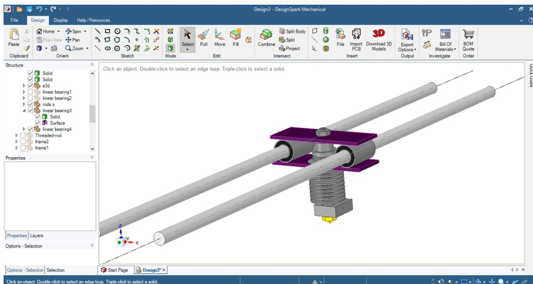
Figure 3.38: 3D design of X axis movement components
