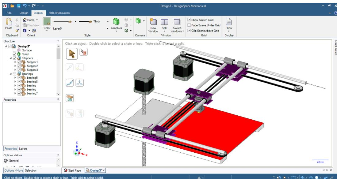
Figure 3.42: Initial concept of the 3D printer without frame
