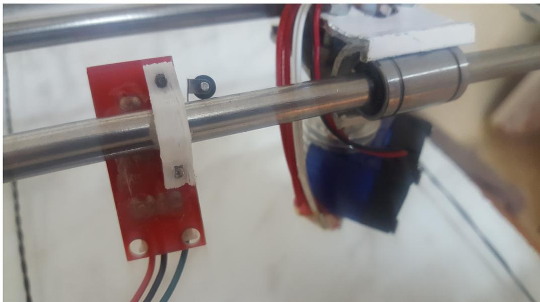
Figure 4.48: after using the 3D printed end-stop holder
