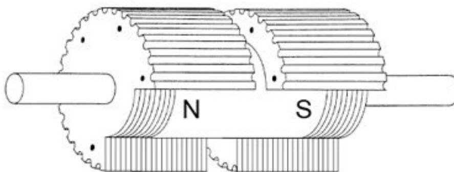
Figure 2.2: Hybrid stepper motor rotor
