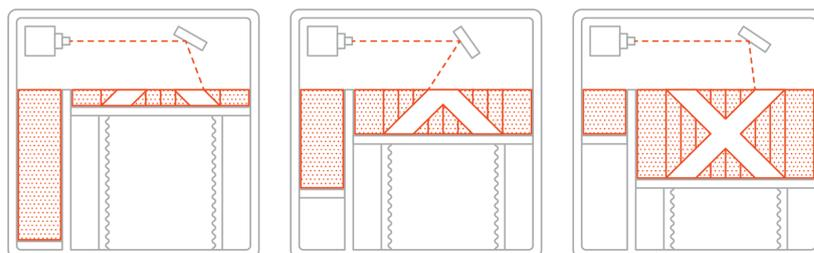
Figure 1.13: 3D printing process Powder Bed Fusion (Metals) based [All19]
