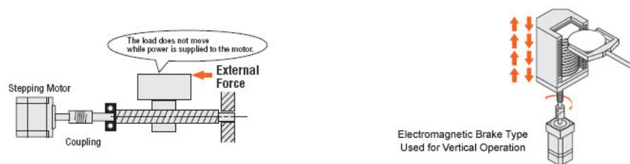
Figure 2.8: Usage examples of holding torque
