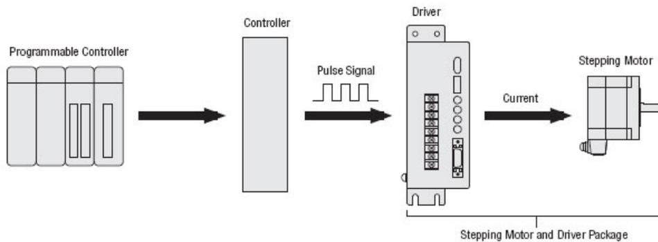
Figure 2.3: Stepper motor control
