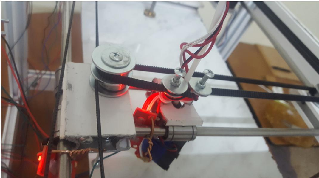
Figure 4.41: End-stops indicating home position at X0 Y0
