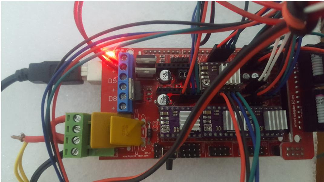
Figure 4.20: Wiring of the 3D printer electronic components
