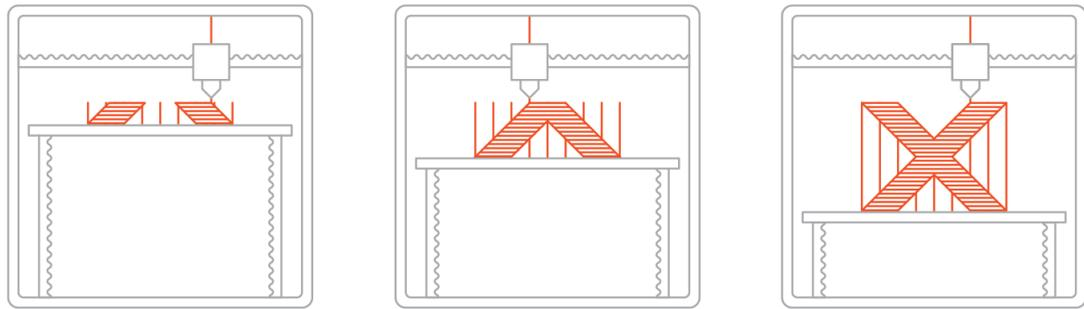
Figure 1.2: 3D Printing Process Material Extrusion based [All19]
