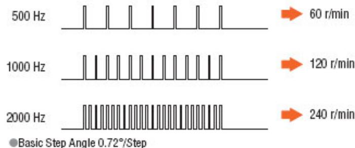
Figure 2.6: The relationship between Rotation Speed and Pulse Speed
