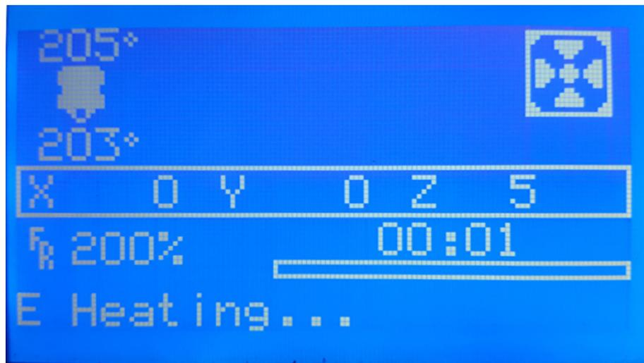
Figure 3.9: 3D printer LCD screen in operation
