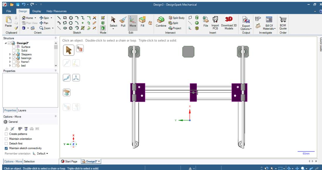
Figure 3.41: Top view of the 3D printer mechanism
