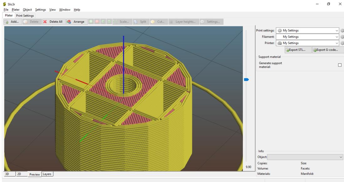
Figure 4.7: Slicing the 3d model using Slic3r
