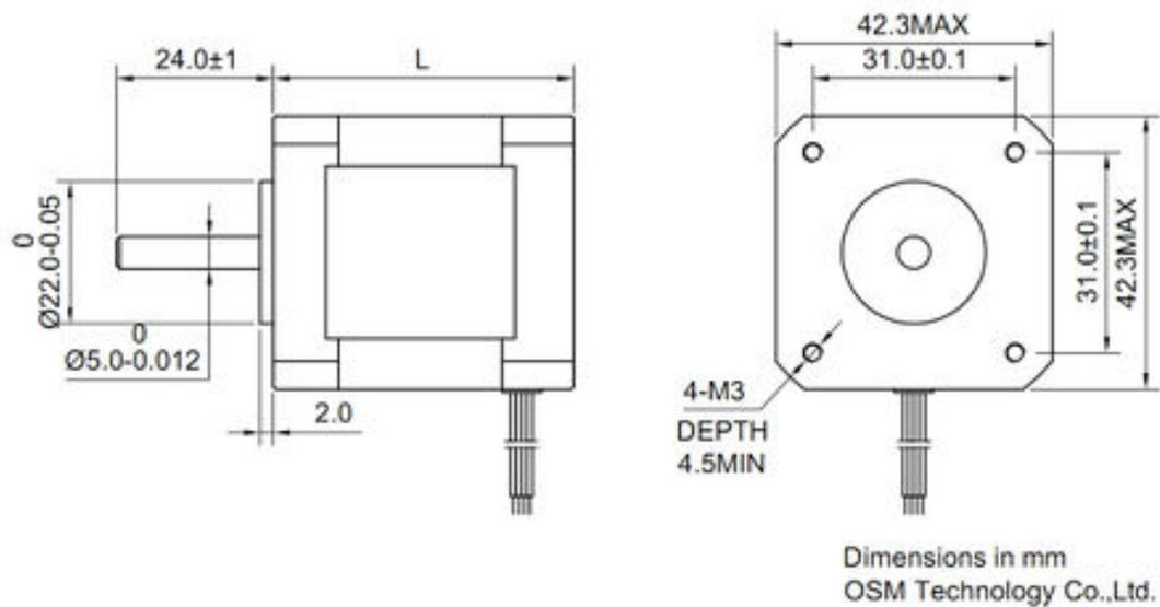
Figure 3.3: Dimensions of NEMA 17 stepper motor[[dim](#)]
