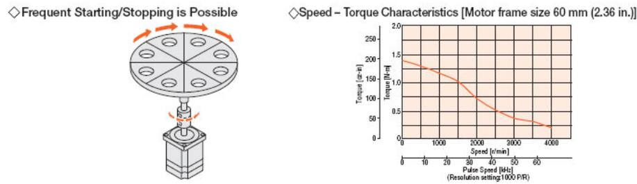
Figure 2.7: Speed torque characteristics
