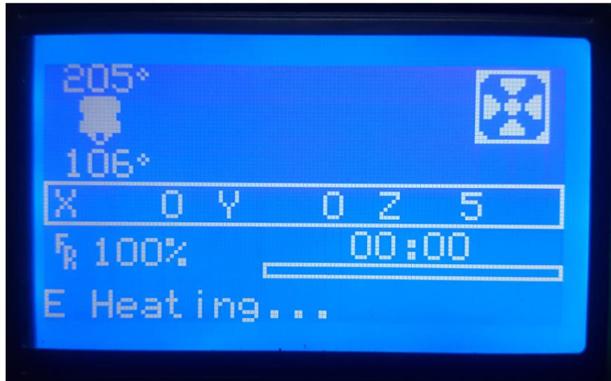
Figure 4.42: Heating the printing head
