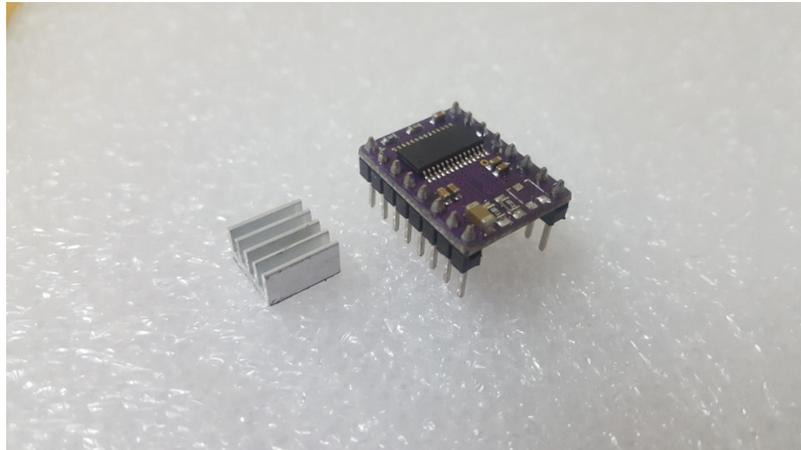
Figure 3.13: stepper driver drv8825 with heat-sink
