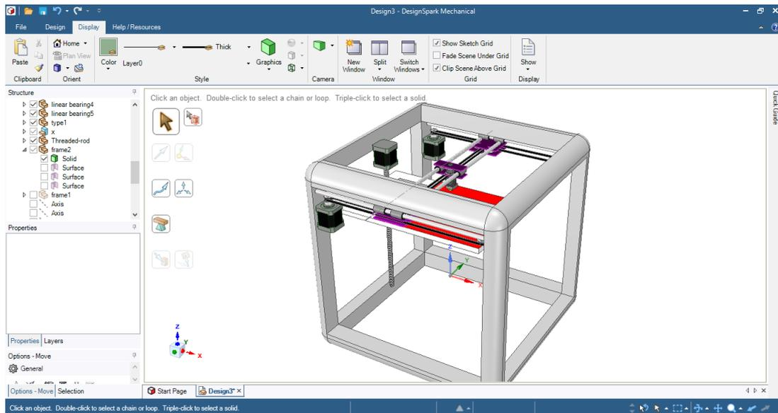
Figure 3.43: initial concept of the 3D printer
