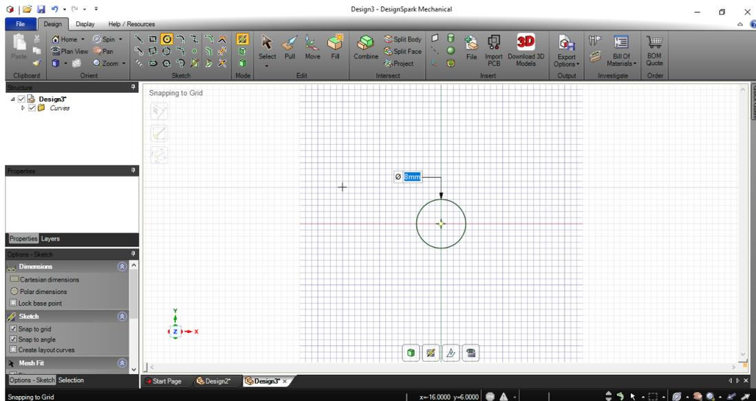
Figure 4.23: sketching circle 8 mm diameter
