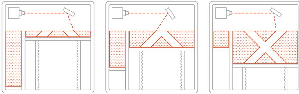
Figure 1.8: 3D printing process Powder Bed Fusion (Polymers) based [All19]
