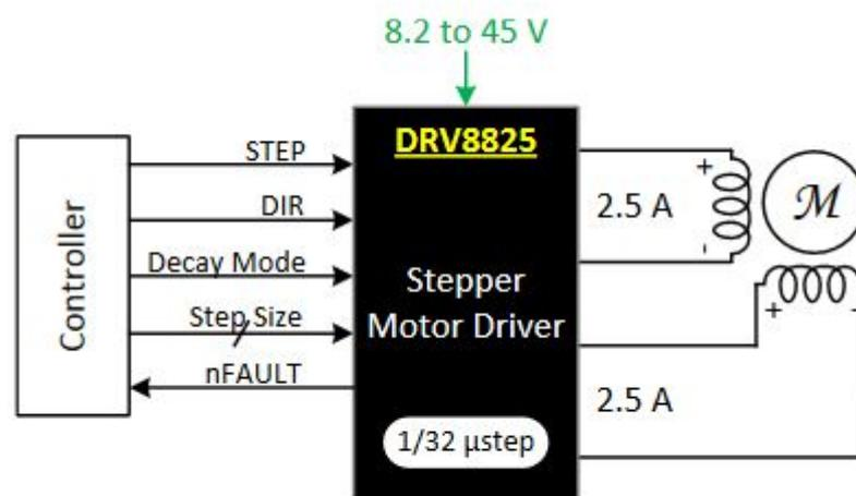
Figure 3.14: Stepper driver simplified schematics [TI11]
