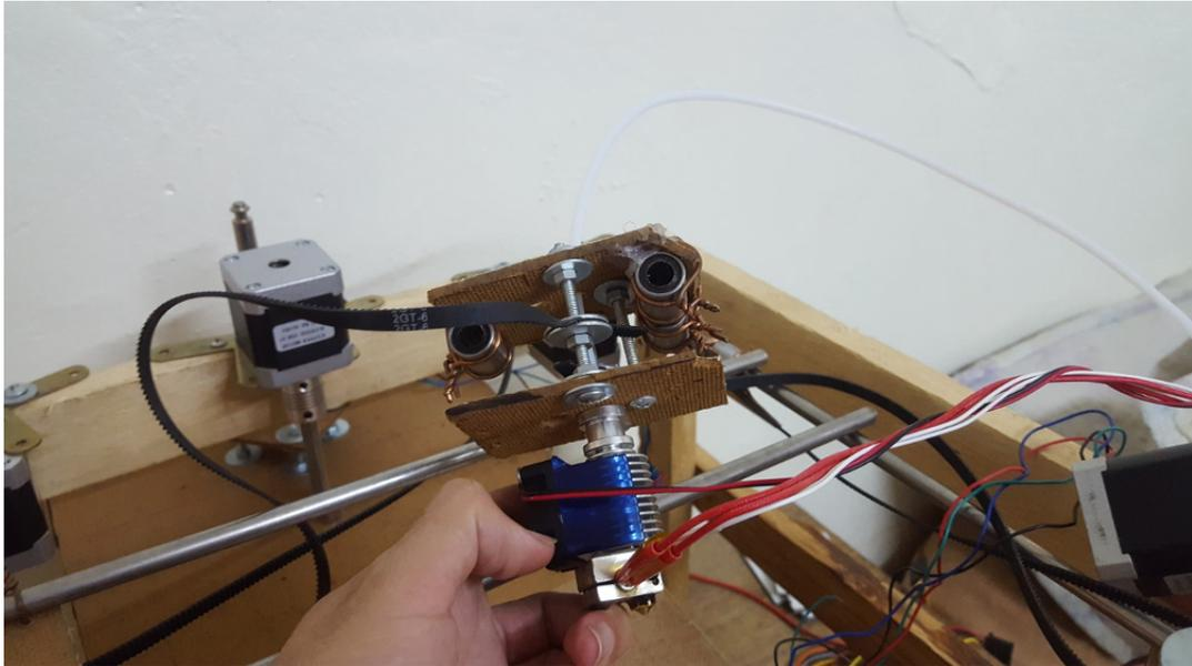
Figure 4.11: disassembly of the wooden frame printer
