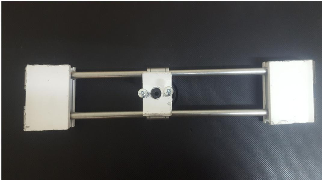
Figure 4.13: top view of the X axis movement components assembled
