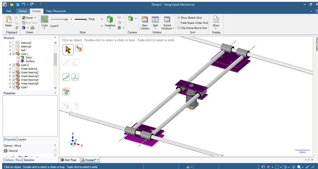
Figure 3.39: 3D design of X and Y axis movement components
