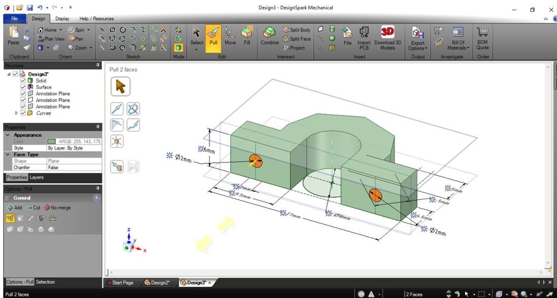
Figure 4.28: making holes for the end-stop holder
