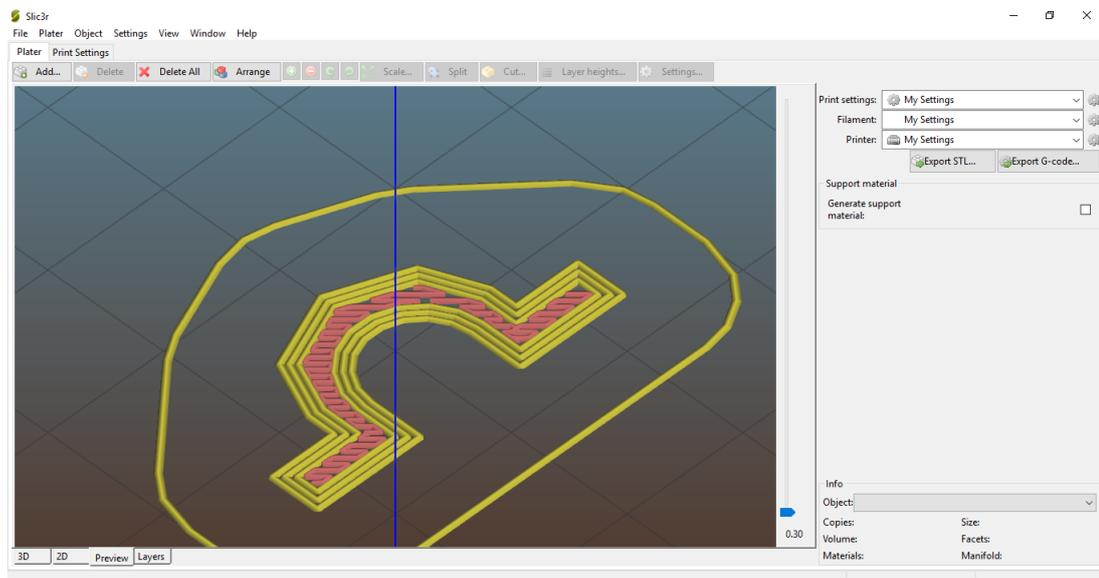
Figure 4.35: first layer for the 3D object in Slic3r
