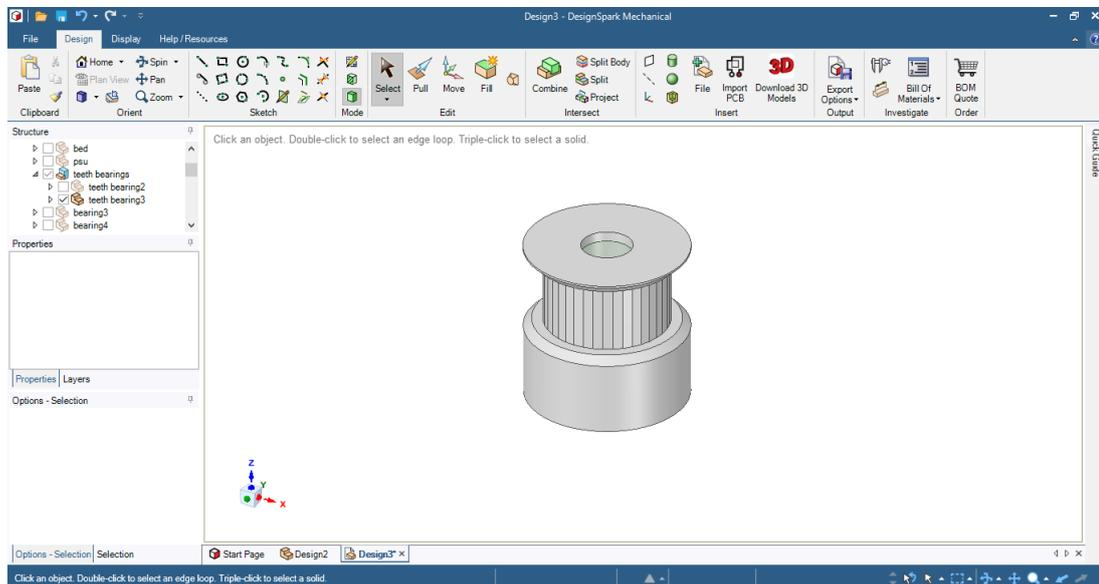
Figure 3.36: 3D design of the of timing belt pulley
