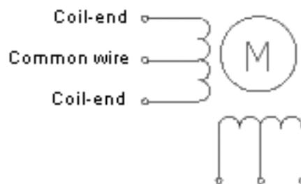
Figure 3.1: Unipolar stepper motor coils
