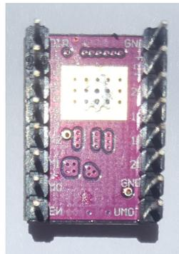
Figure 3.16: stepper driver back view
