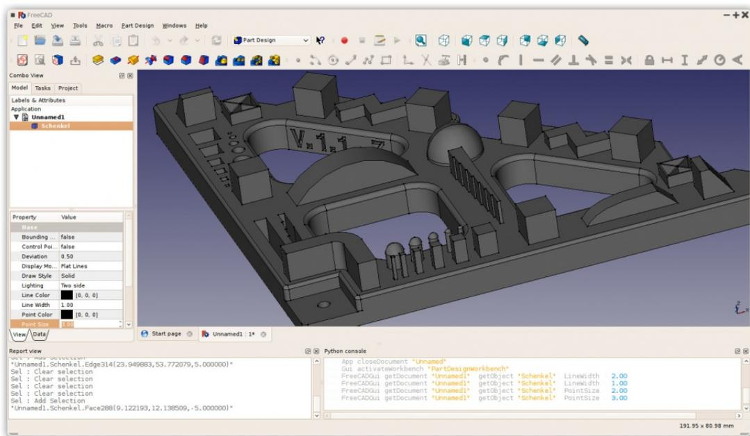
Figure 3.21: User interface of the CAD software FreeCAD[fre]
