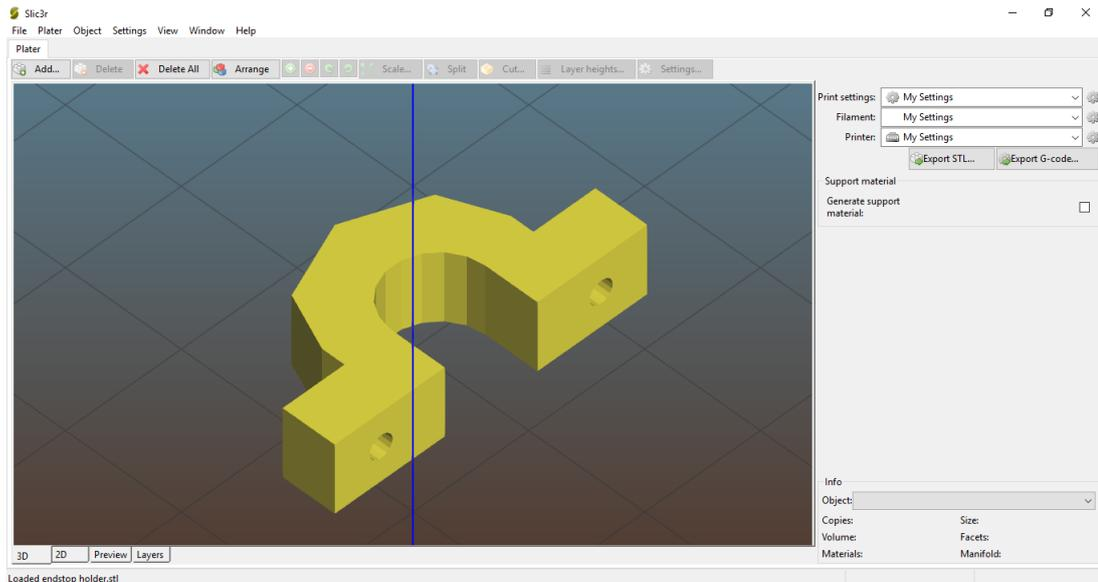
Figure 4.31: importing the model to Slic3r
