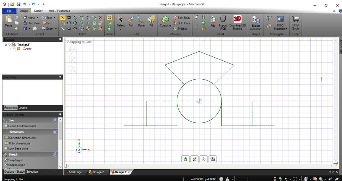
Figure 4.25: sketching the geometry of the end-stop holder
