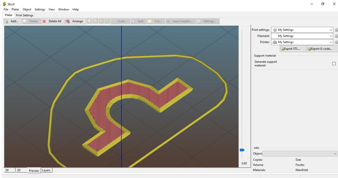
Figure 4.36: second layer for the 3D print in Slic3r
