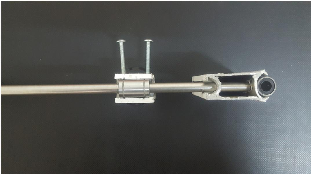
Figure 4.14: side view of the X axis movement components assembled
