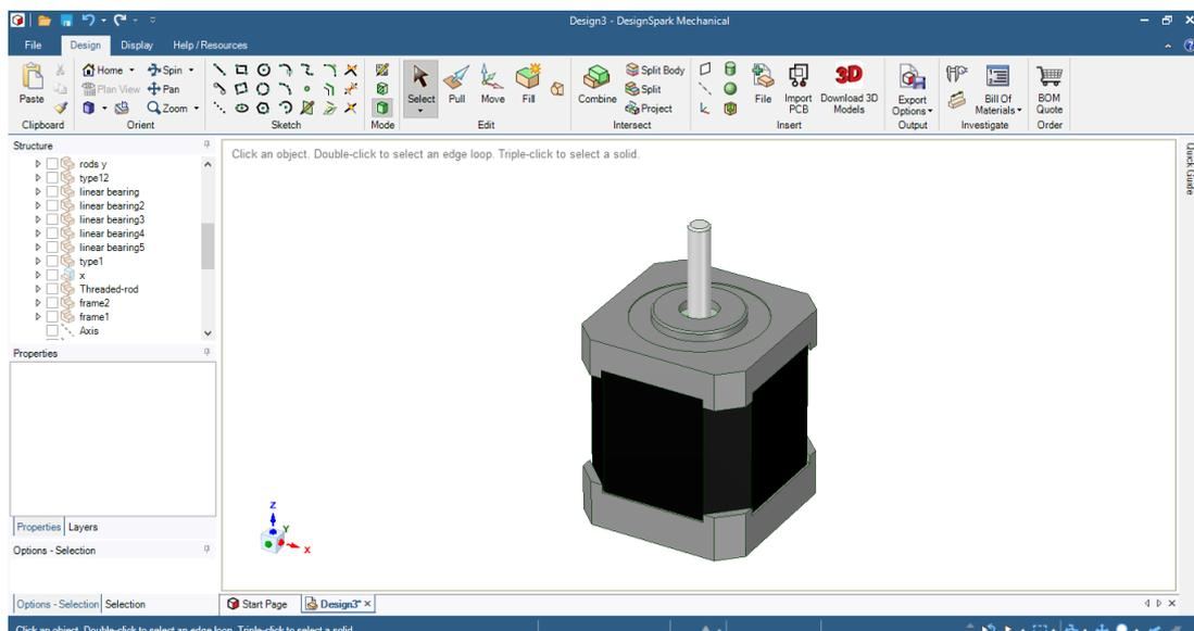
Figure 3.31: 3D design of a stepper motor
