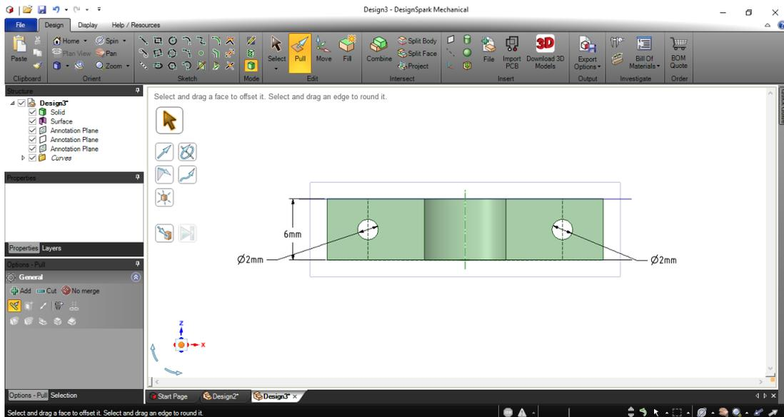
Figure 4.29: side view of the end-stop holder
