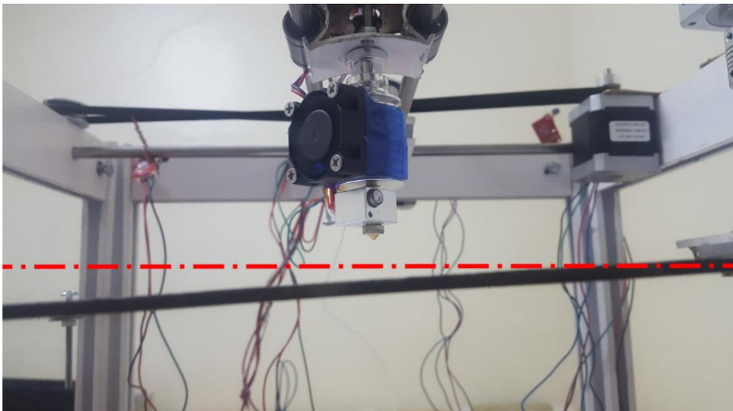
Figure 4.21: Tilted printing base side view
