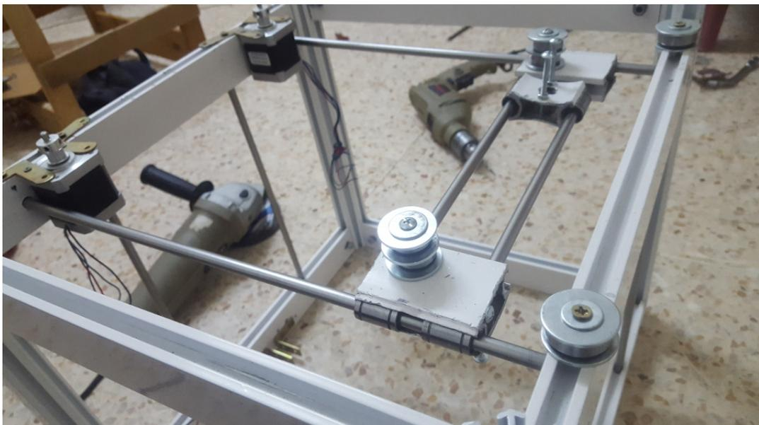
Figure 4.15: X and Y movement components
