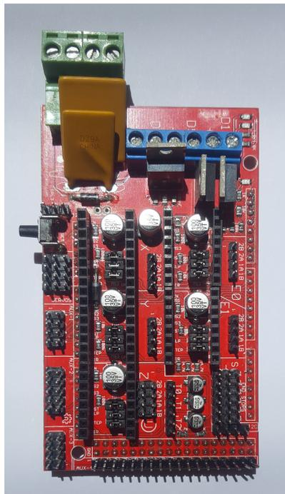
Figure 3.12: Picture of The RAMPS board
