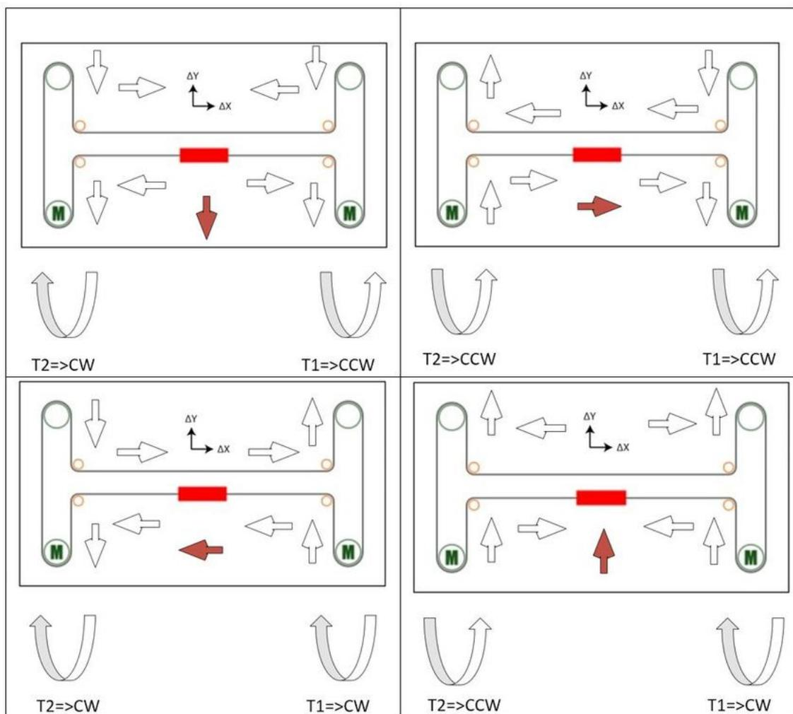
Figure 2.1: Movement analysis in the H-bot mechanism [hbo]
