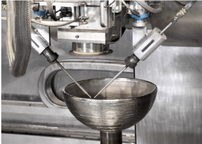
Figure 1.14: Electron Beam Melting [[typ18](#)]
