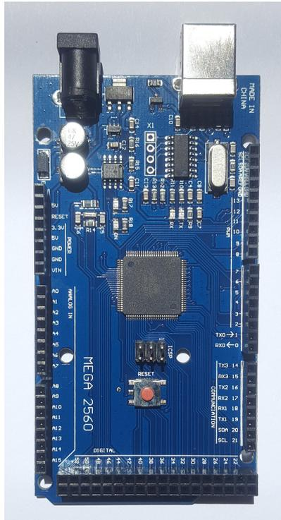
Figure 3.10: Picture of the ARDUINO mega board
