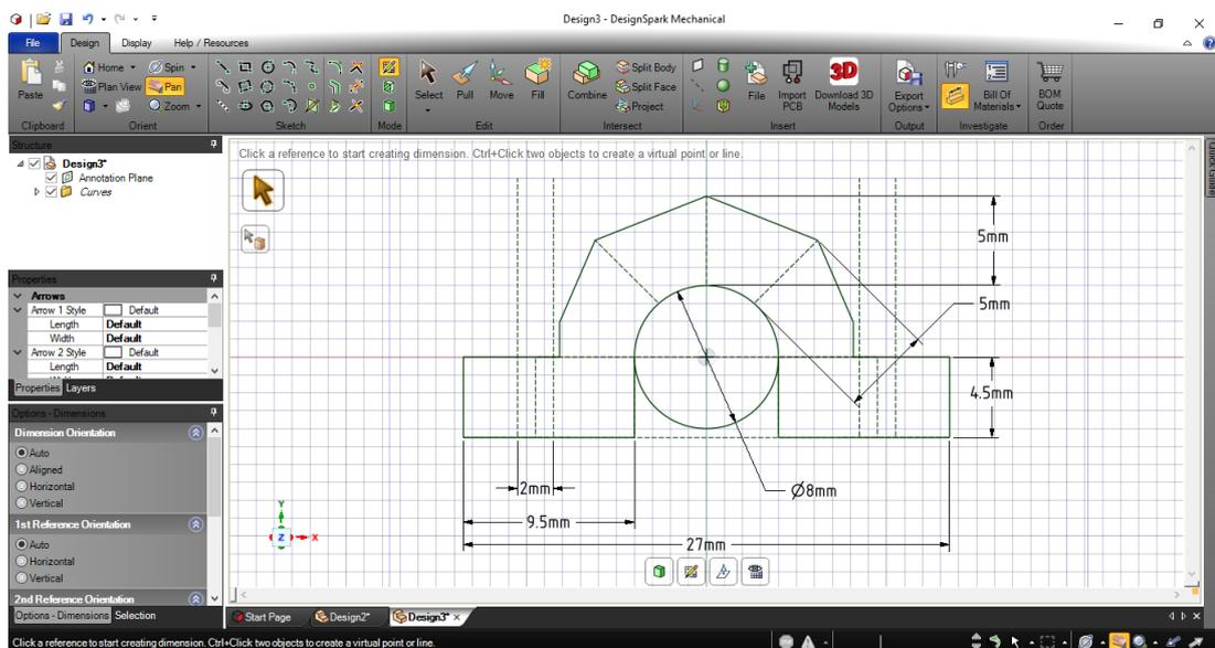
Figure 4.26: final geometry of the end-stop holder with lengths
