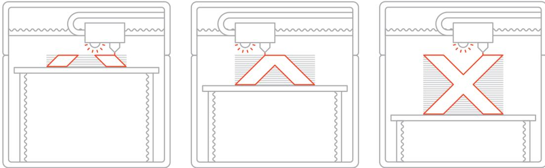
Figure 1.10: 3D printing process Material Jetting based [All19]
