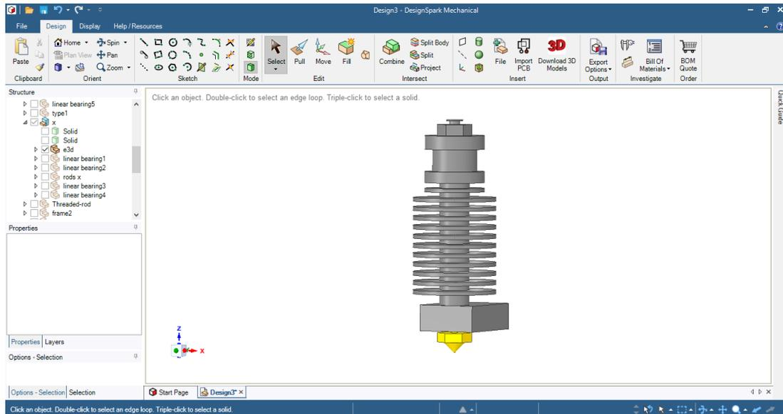
Figure 3.32: 3D design of the hot-end
