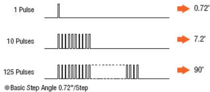
Figure 2.5: The relationship between the stepper motor's angle of rotation and pulse number
