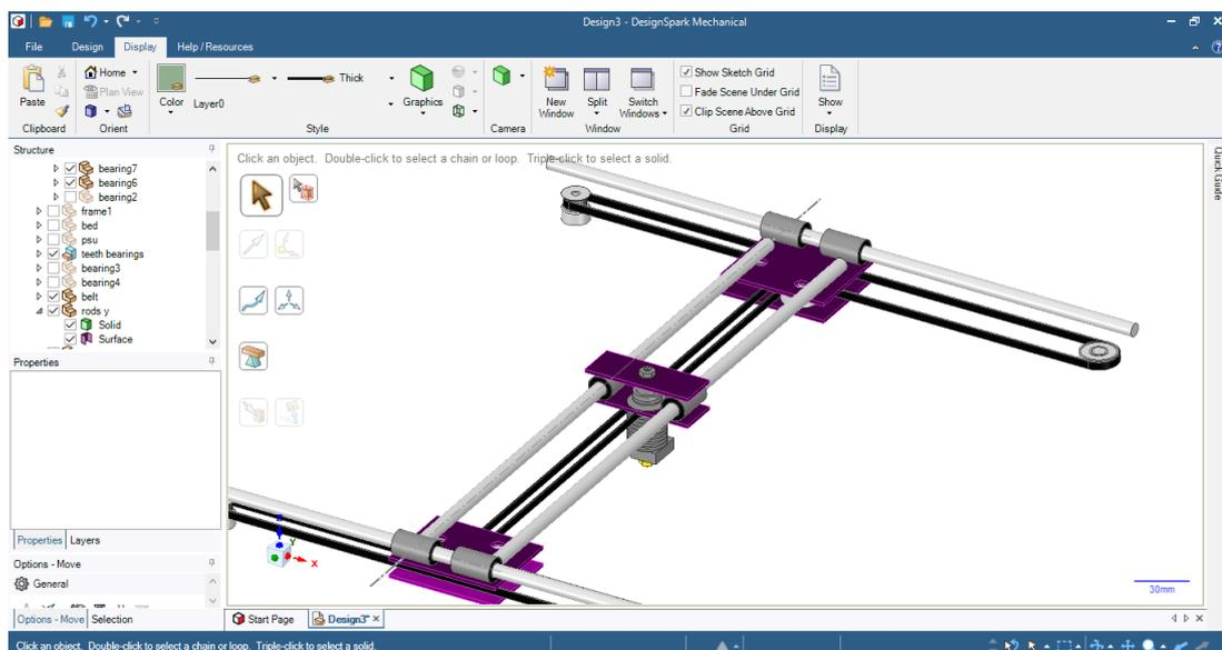
Figure 3.40: Bearings and belt installation
