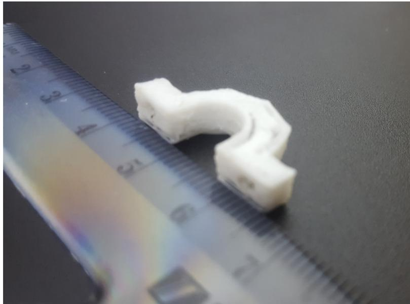
Figure 4.46: end-stop holder dimension accuracy check
