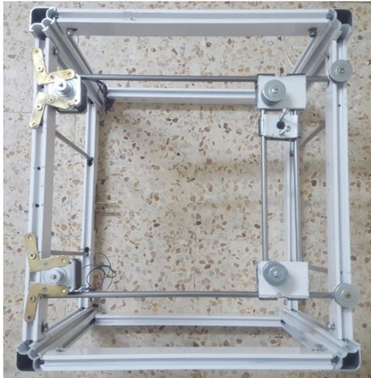
Figure 4.16: top view of the 3D printer after assembling metal parts
