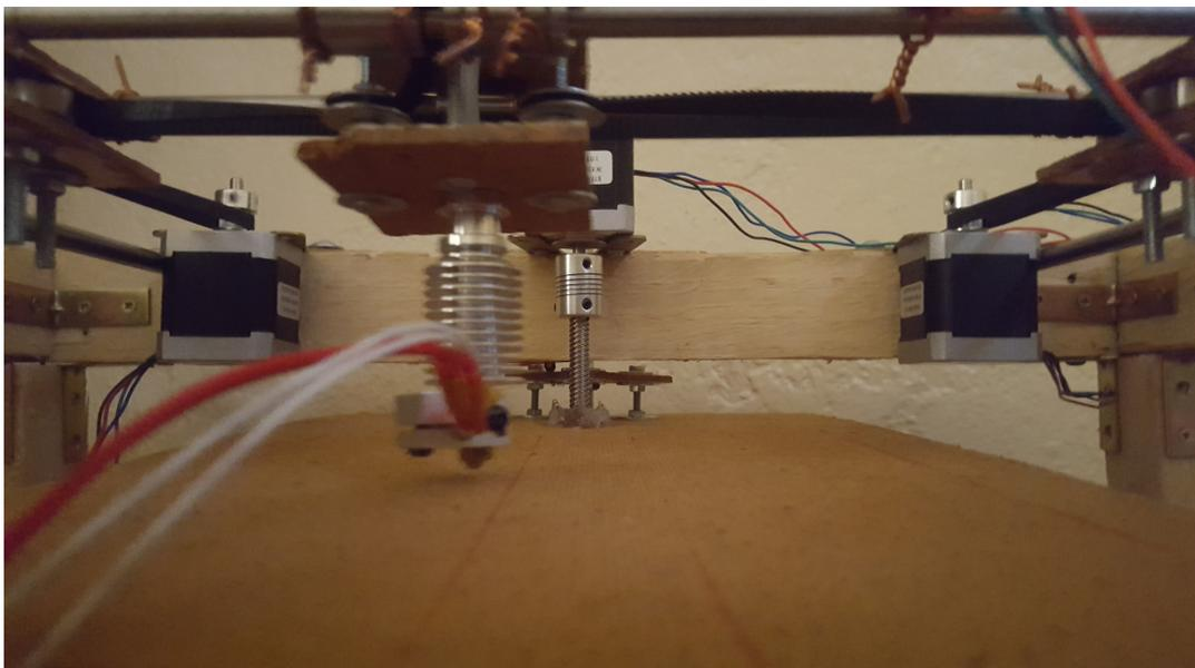
Figure 4.3: After mounting the base and the z axis
