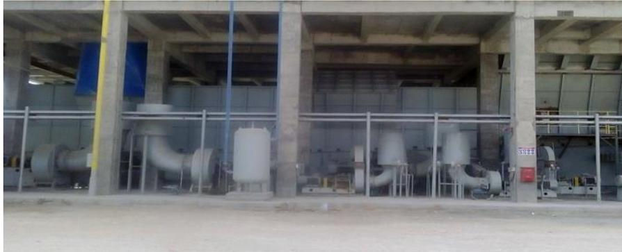
Figure I.12: Grid Cooler.
