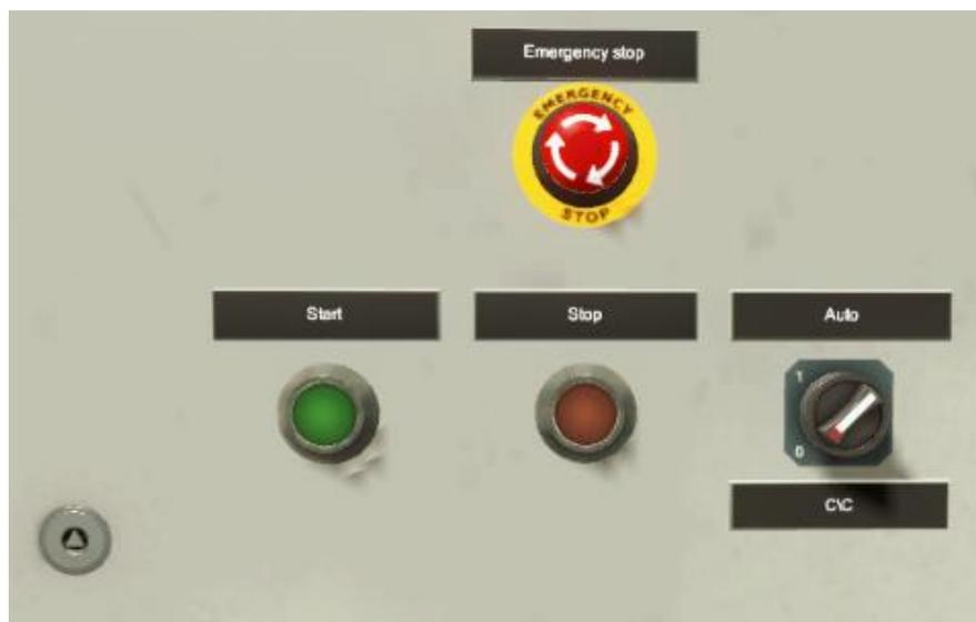
Figure III.1: Control panel.
