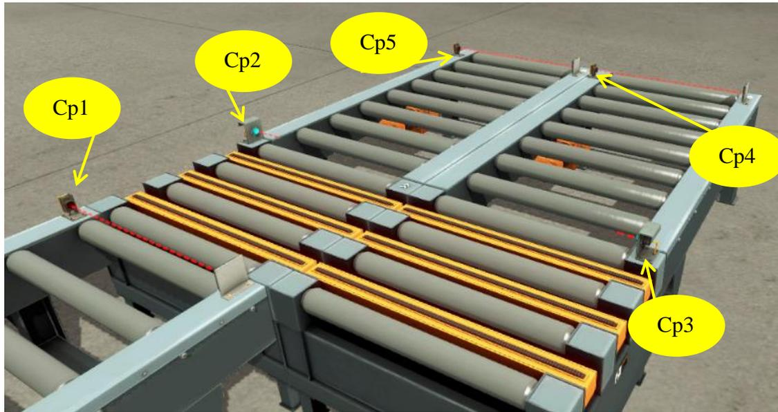
Figure III7: Position of the sensors in the Chain Transfer.
