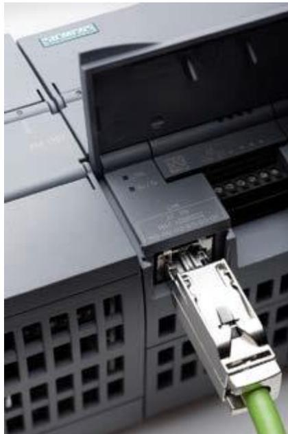
Figure II.18: PROFINET connection.
