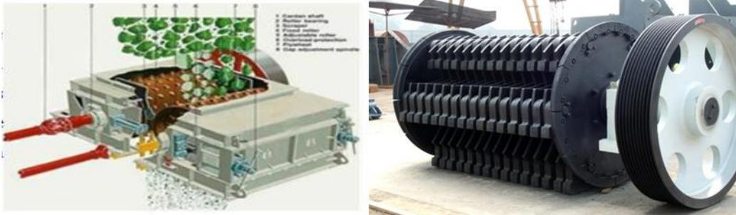
Figure I.4: Hammer crusher.
