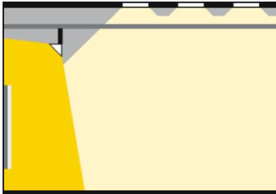
Fig (I-14) Directional lighting for the wall, diffuse lighting for the room
