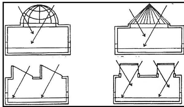
Fig (I-13) Types of roof openings source: (neufert, 2010)
