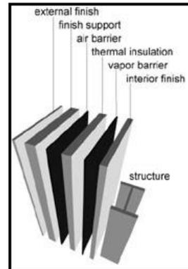
Fig (I-2) the layers of wall
