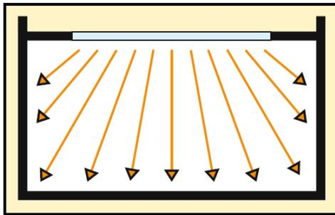
Fig (I-11) Daylight incidence from above through a luminous ceiling source: (Licht, 2018)
