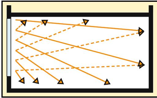
Fig (II-9) Daylight incidence from the side through a window source: (Licht, 2018)
