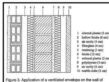
Figure 3. Application of a ventilated envelope on the wall of
