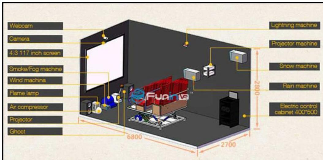
Fig (I-21) the components of 7D cinema
