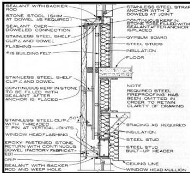
Fig (I-3) the layers of the new wall
