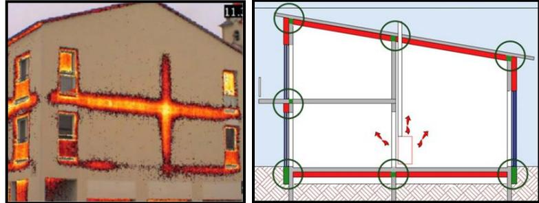
Fig (I-6) the thermal bridges
