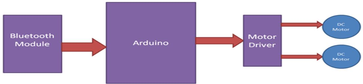
figure IV.14. Block diagram Bluetooth control
