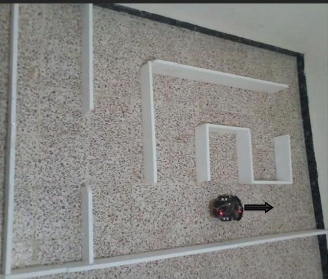
figure IV.45. The robot is now in the cells (3,3). In these cells, the robot does not find a new wall. So the update cell values do not cause any changes in the value of the cell. Then the robot doing the movement to neighboring cells that have the smallest value, ,the robot now go to (3,3).
