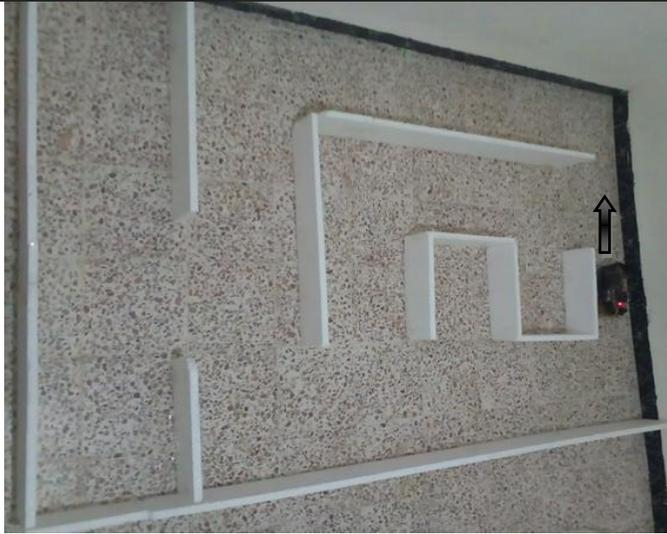
figure IV.48. the robot is now in a cell (2,5). In this position, the robot finds a new wall on the west side. After the robot to update the value of the cell, then the cell (2, 4) will change the value. So that the robot will move to a neighboring cell that has the smallest value ,the robot now go to (1,5).
