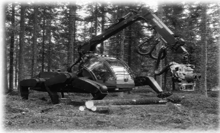
Figure I.1. Driven Walking Robot [5]
