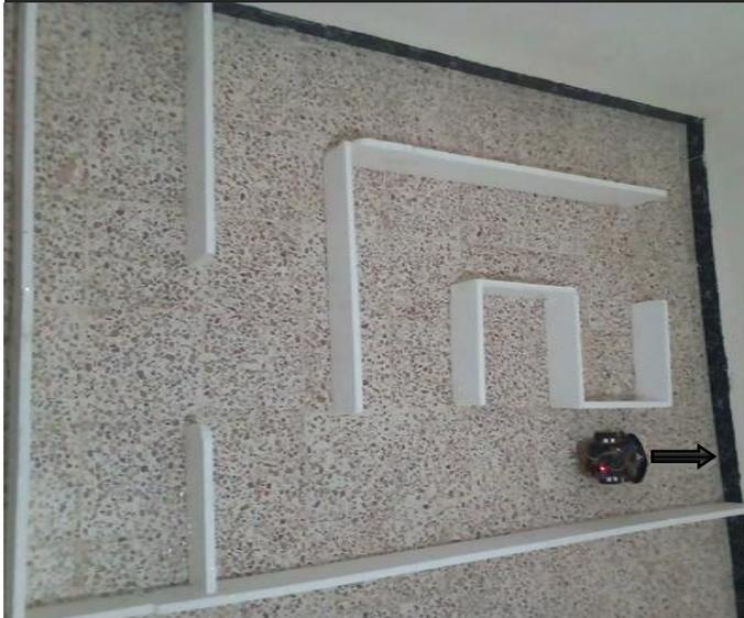
figure IV.46. the robot is now in a cell (3,4). In this position, the robot finds a new wall on the west side. After the robot to update the value of the cell, then the cell (3,4) will change the value. So that the robot will move to a neighboring cell that has the smallest value, is cell but in this situation there is two cells equal south and north we set the Priority always at north ,the robot now go to (3,5).
