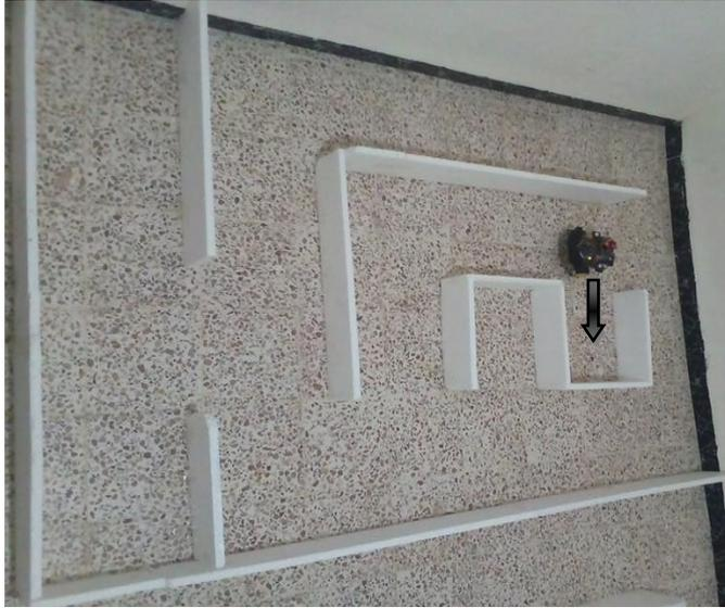
figure IV.50. the robot is now in the cells (1,4). In these cells, the robot does not find a new wall. So the update cell values do not cause any changes in the value of the cell. Then the robot doing the movement to neighboring cells that have the smallest value, ,the robot now go to (2,4).
