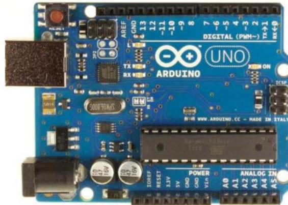
Figure II.2. Arduino Uno [25]
