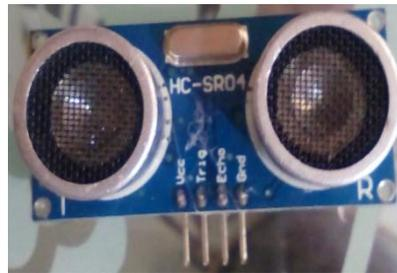
figure IV.7.Ultrasonic Sensors HC-SR04
