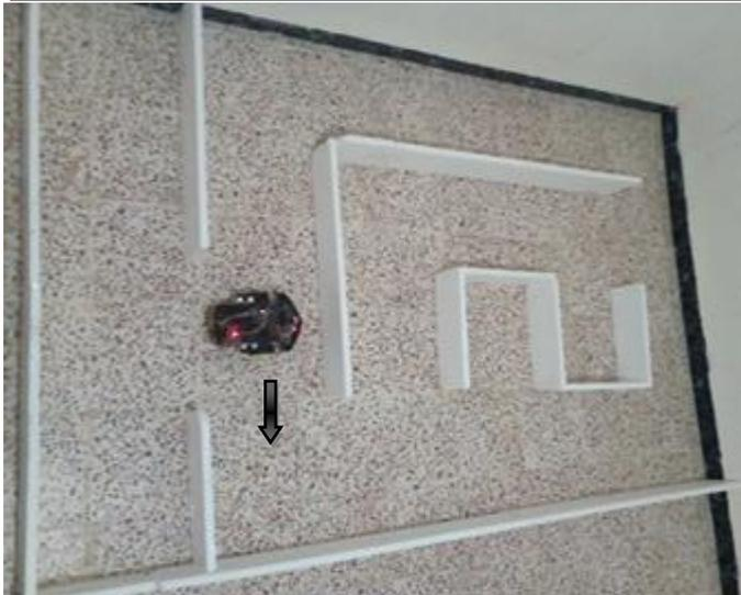
figure IV.42. The robot is now in a cell (2,1). In this position, the robot finds a new wall on the north side. After the robot to update the value of the cell, then the cell (2, 1) will change the value. So that the robot will move to a neighboring cell that has the smallest value, is cell but in this situation there is two cells equal East and west we set the Priority always at east ,the robot now go to (3,1).
