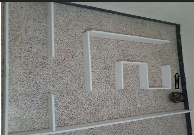
figure IV.47. the robot is now in the cells (3,5). In these cells, the robot does not find a new wall. So the update cell values do not cause any changes in the value of the cell. Then the robot doing the movement to neighboring cells that have the smallest value, ,the robot now go to (2,5).
