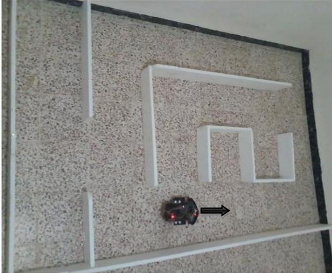
figure IV.44. the robot is now in the cells (3,2). In these cells, the robot does not find a new wall. So the update cell values do not cause any changes in the value of the cell. Then the robot doing the movement to neighboring cells that have the smallest value ,but in this situation there is two cells equal north and west we set the Priority always at north ,the robot now go to (3,3).
