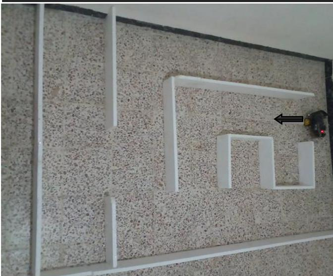
figure IV.49. the robot is now in the cells (1,5). In these cells, the robot does not find a new wall. So the update cell values do not cause any changes in the value of the cell. Then the robot doing the movement to neighboring cells that have the smallest value, ,the robot now go to (2,4).
