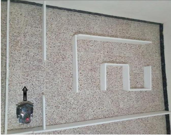
Figure IV.40. The robot is in the cell (3, 0). The robot finds a new wall on the east side. Then the robot will update the value of a cell by placing cells (2, 4) as the destination cell, so the search is done on cell lines (3, 0) to the cell (2, 4). Then the robot will move to a neighboring cell that has the smallest value that the cells (2, 0).
