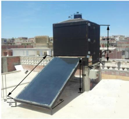
**Fig (II-36):** The experimental solar dryer.
