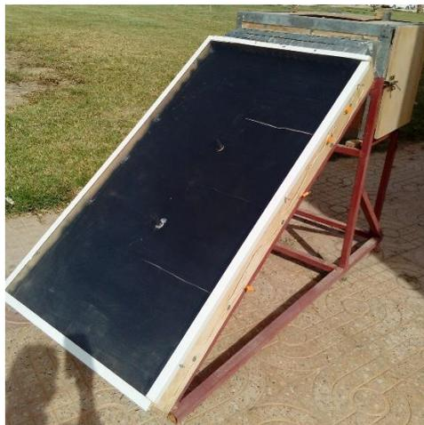
Fig (III-3): Experimental setup (solar collector with drying chamber).
