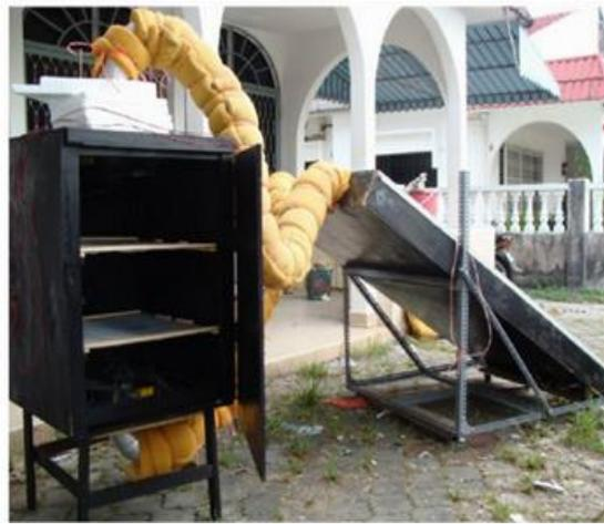
**Fig (II-15):** Picture of indirect forced circulation solar drying thermal system.
