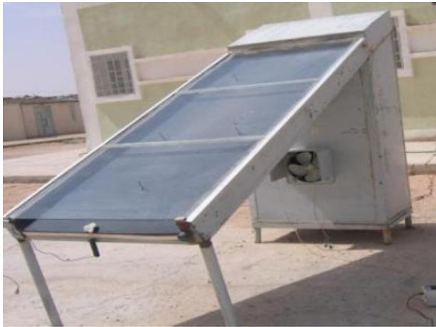
**Fig (II-27):** Schematic of the drying system.
