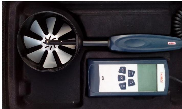
**Fig (III-14):** A digital anemometer (Model KIMO-LVA).
