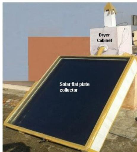
**Fig (II-30):** pictorial view of the solar drying system.
