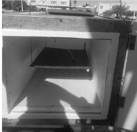
**Fig (III-6):** Support of the drying product.
