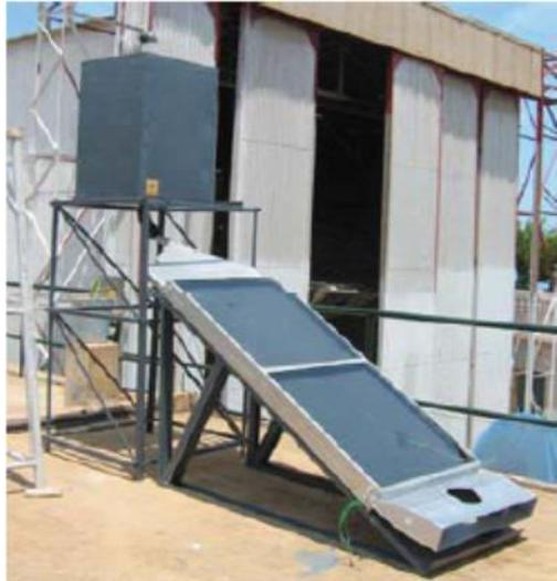
**Fig (I-11):** The indirect solar dryer [19].
