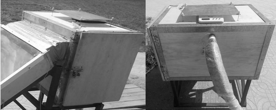
**Fig (III-4):** Experimental setup of drying chamber.
