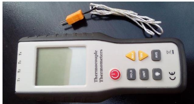
**Fig (III-11):** A thermocouples type k.
