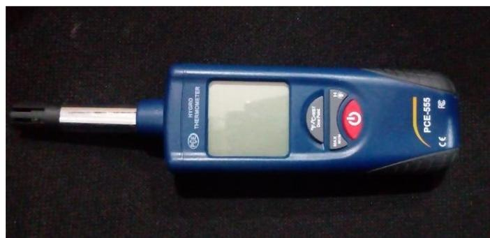
**Fig (III-12):** Hygrometer (Model PCE-555).
