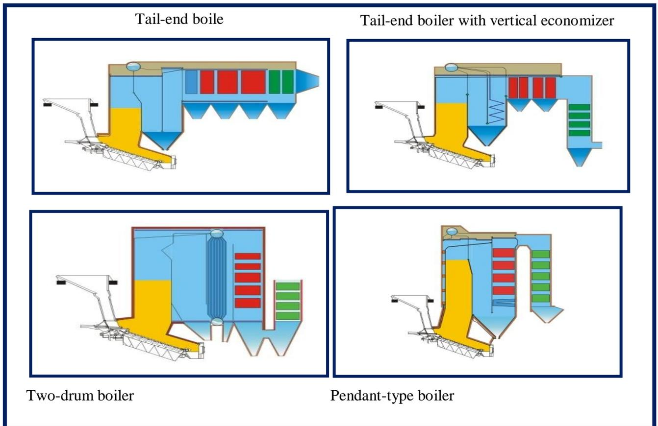
**Figure 40:** Various boiler designs. Source: [MAR 13]
