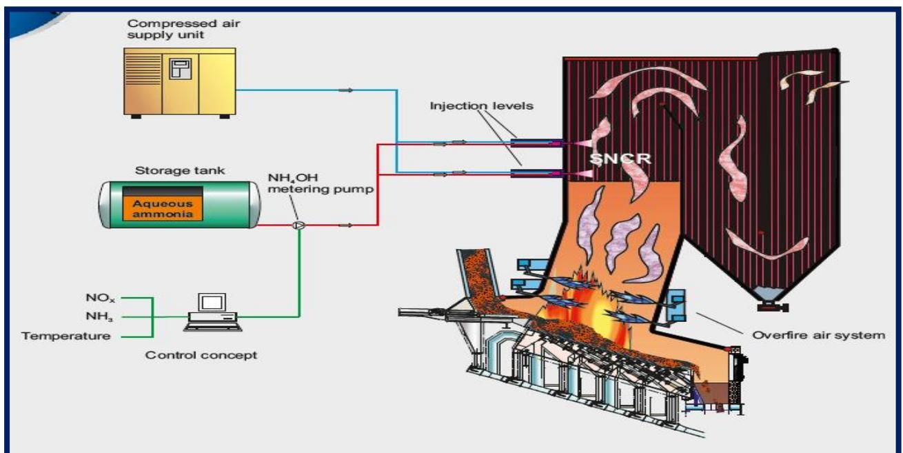
Figure 39: SNCR system Source: [MAR 13]
