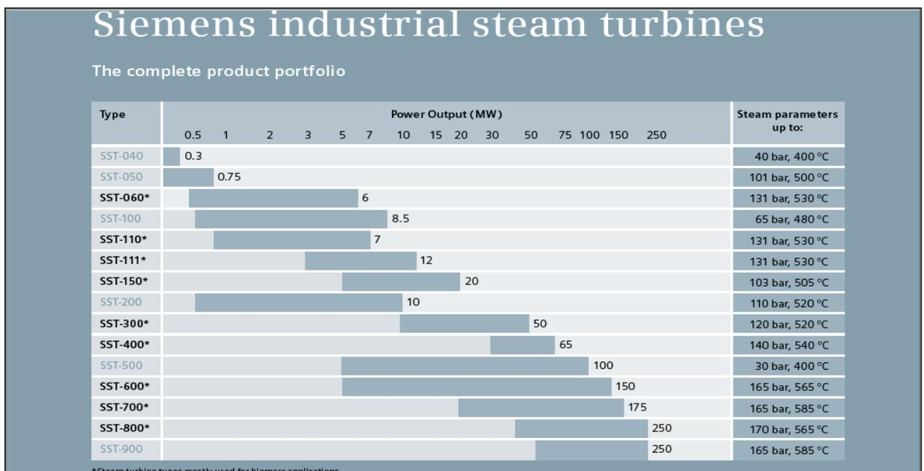
Figure 20: Siemens industrial steam turbines. Source: [SIE 17]
