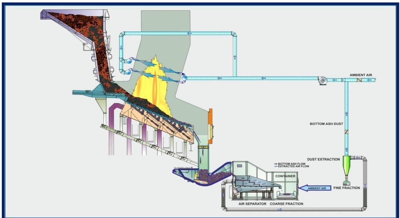
**Figure 42:** Dry discharge system. Source: [MAR 13]
