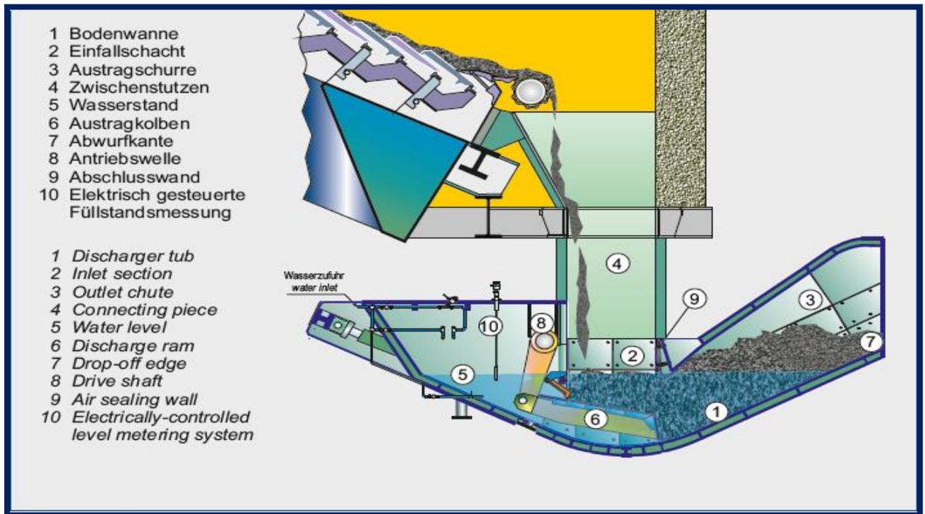
Figure 38: discharge invention. Source: [MAR 13]
