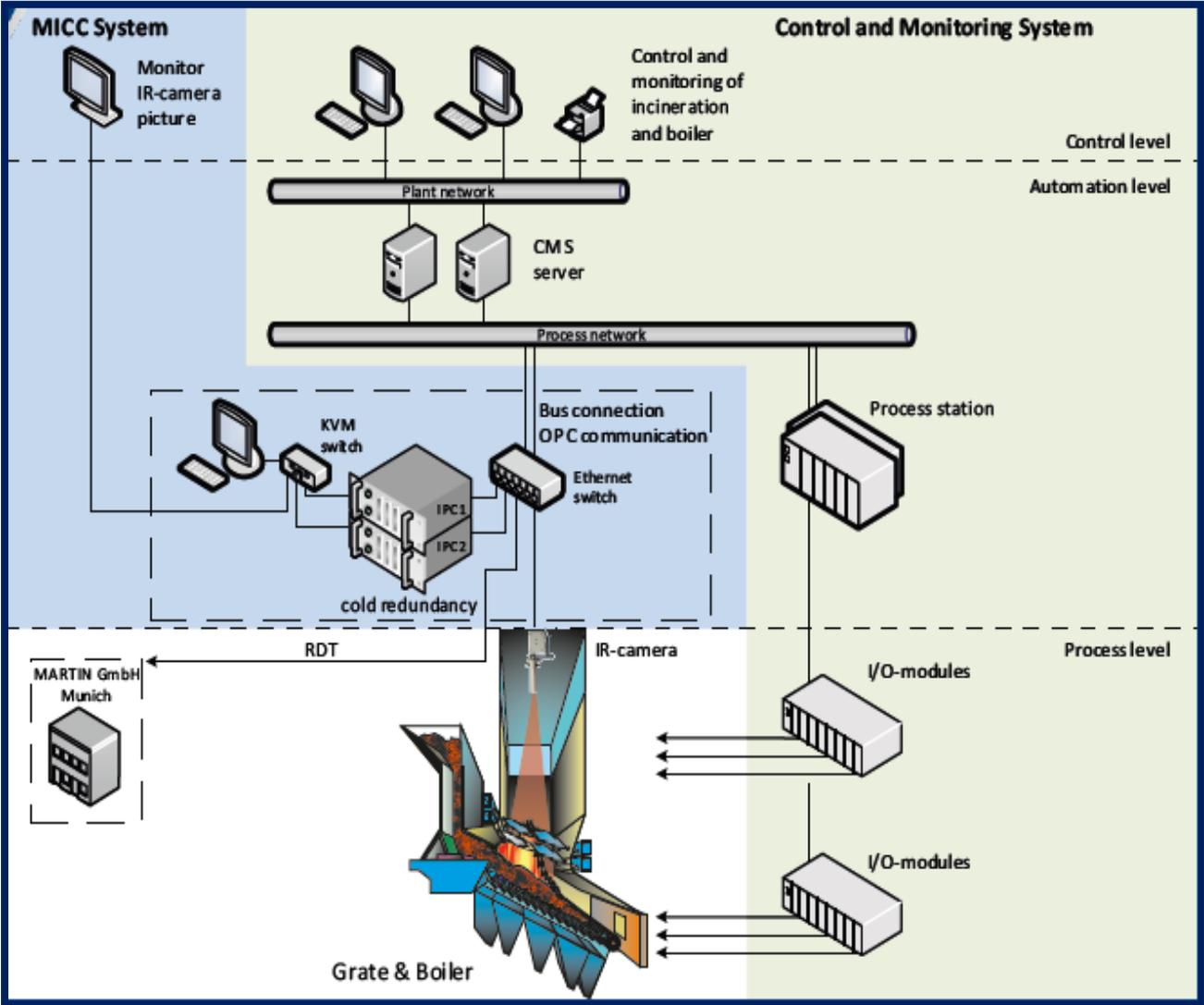
Figure 41: MICC - MARTIN Infrared Combustion Control. Source: [MAR 13]
