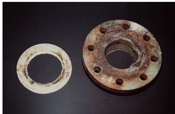
*Figure.I.5:la corrosion caverneuse[10]*
