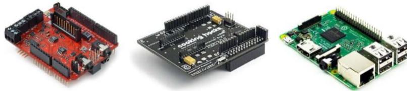
Figure 4.3.5: From left to right: -The E-HP, -The Connection bridge, -Raspberry Pi3 B
