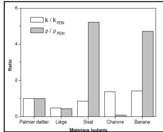
Figure 3.52: Comparison of density and thermal conductivity of date palm wood with other
