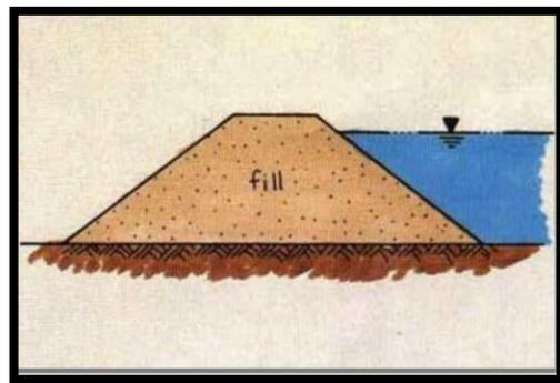
Figure 1.3: Making Embankment
