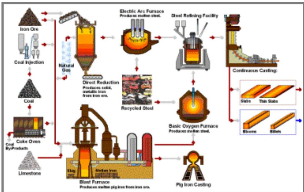
Figure 1.7: Iron smelting
