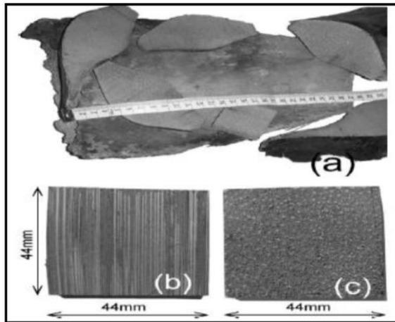
Figure 3.51: petioles used (a); sample with fibers.
