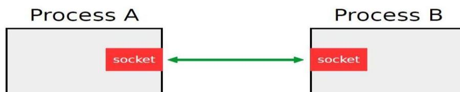
**FIGURE 2.1:** Socket End on Each Process.
