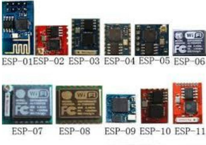
Fig .II.14 ESP8266 Boards
