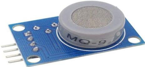
Fig.III.3 MQ9 Carbon Monoxide Sensor (CO)
