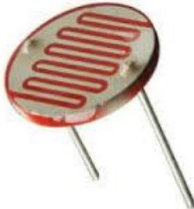
**Fig.III.5** Light Dependent Resistor LDR
