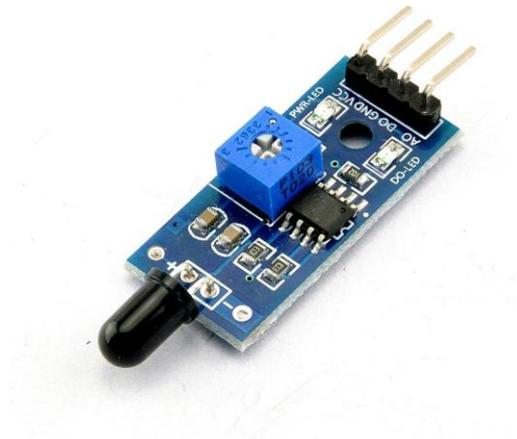
**Fig.III.4** Flame Sensor
