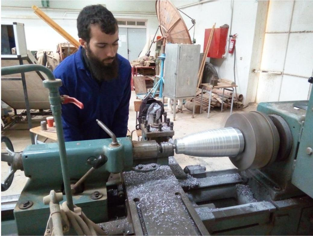
**Figure E.1.** I was working on the nose cone in milt machine.
