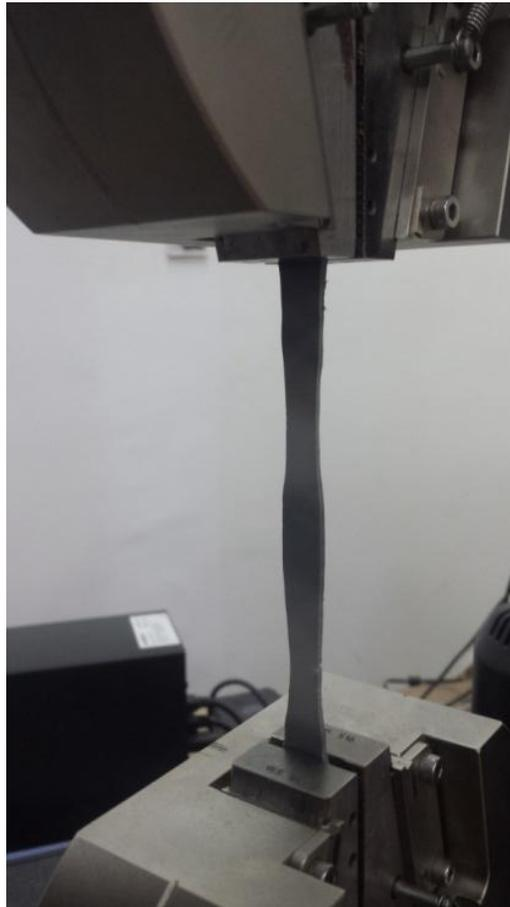
**Figure VIII.4.** Tensile experiment on PVC spicement.
