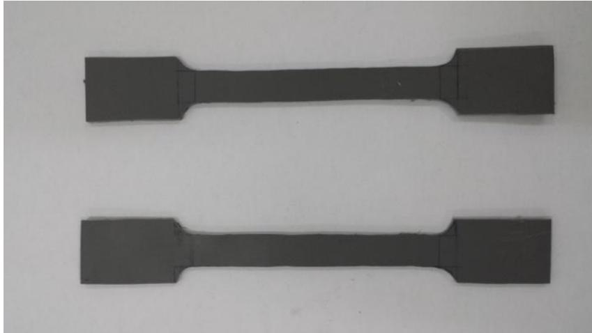
**Figure VIII.3.** PVC (polyvinyl chloride) spicement.
